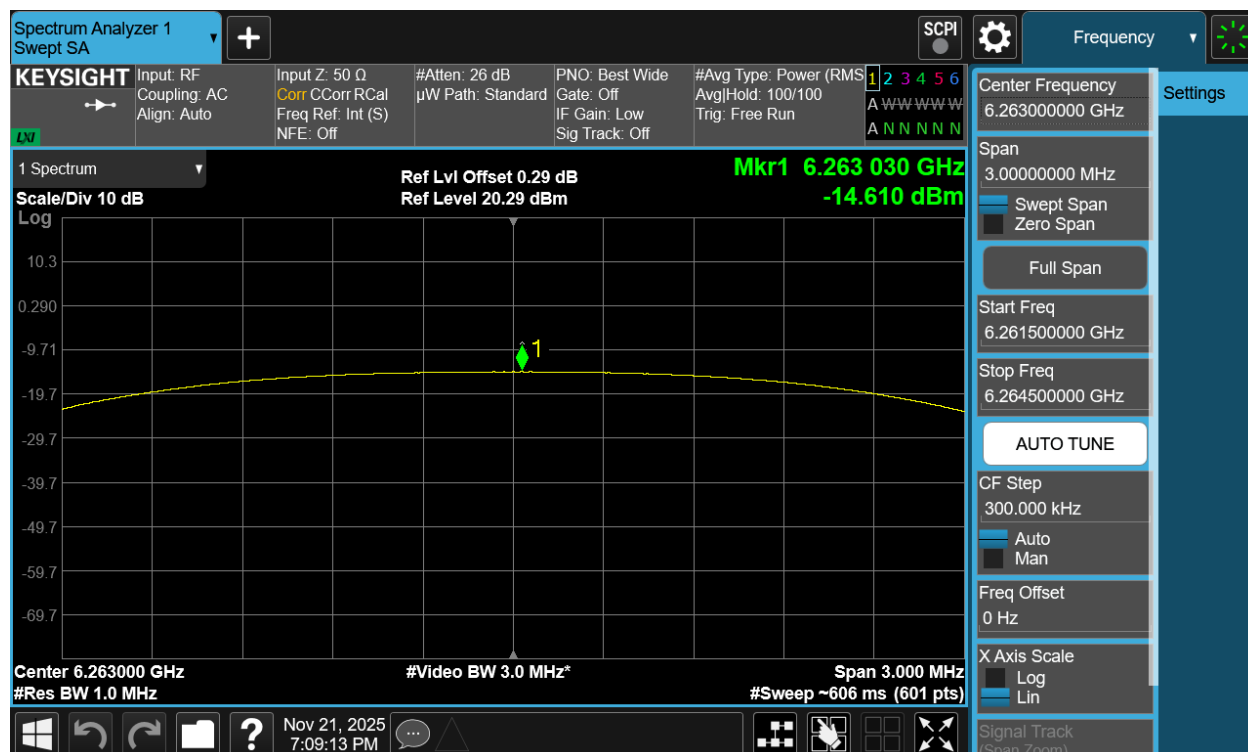
Plot 7-217. PSD TxBF Diversity Antenna 1b (NB UNII HDT4, iPA – 6263MHz)
