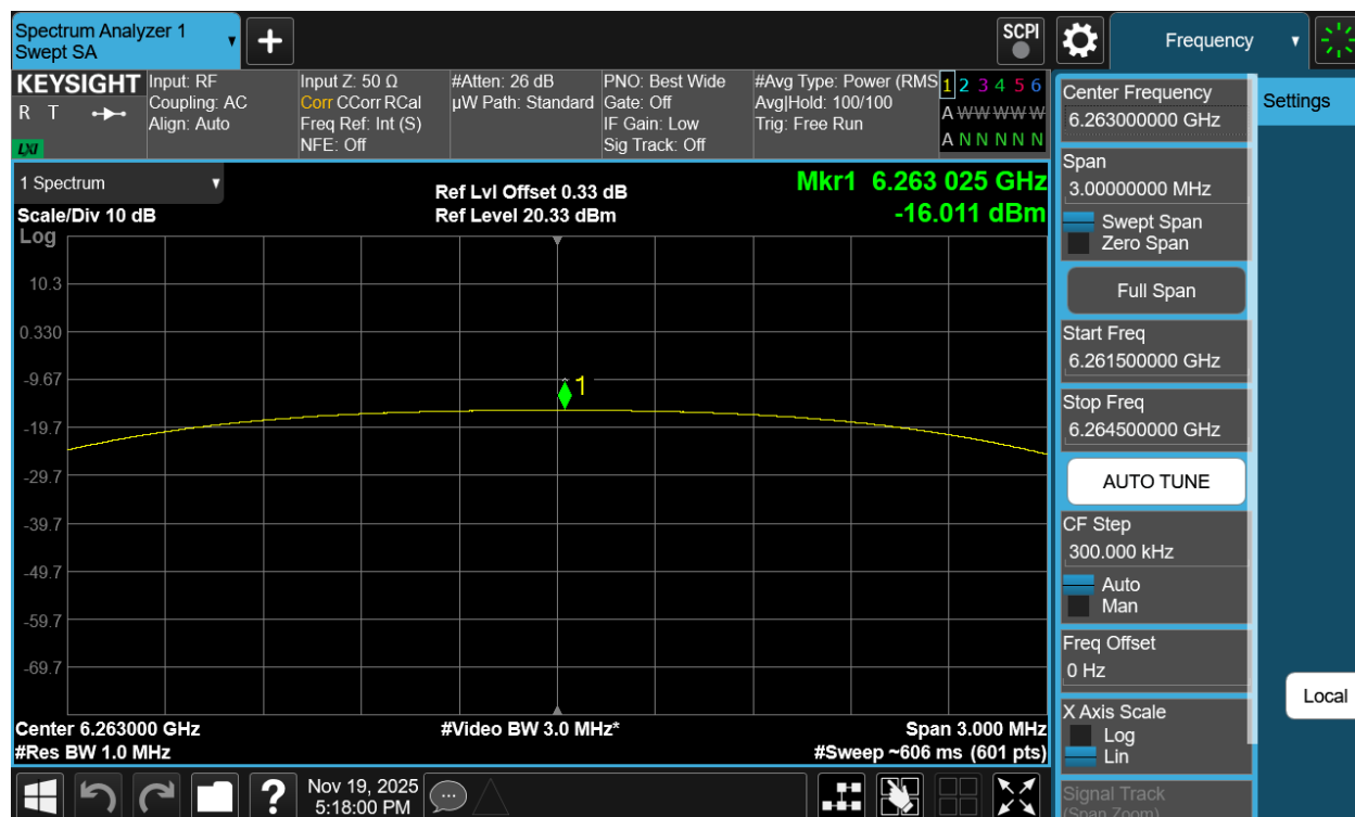
Plot 7-214. PSD Tx BF Diversity Antenna 5T (NB UNII HDT4, ePA – 6263MHz)
