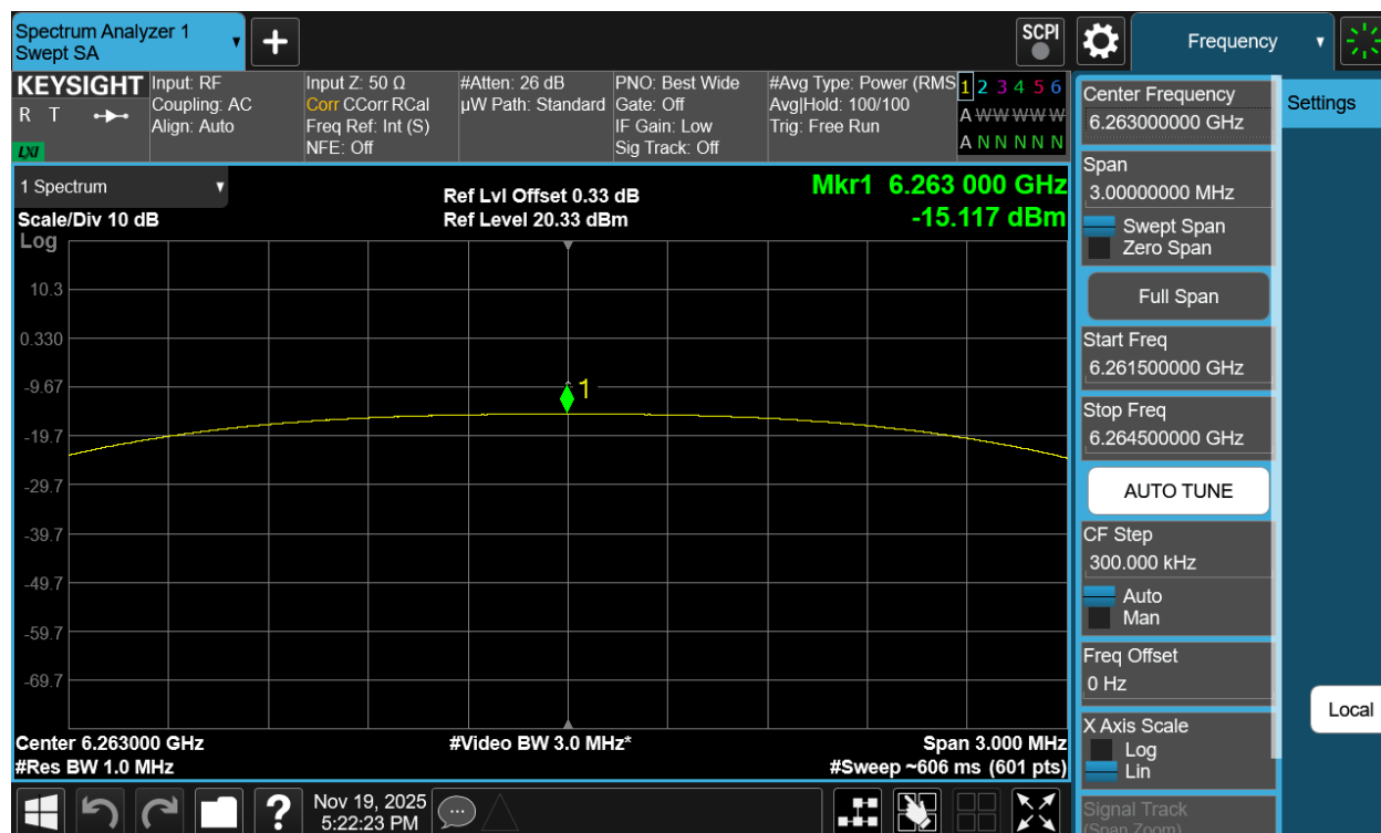
Plot 7-216. PSD TxBF Diversity Antenna 5T (NB UNII HDT4, iPA – 6263MHz)
