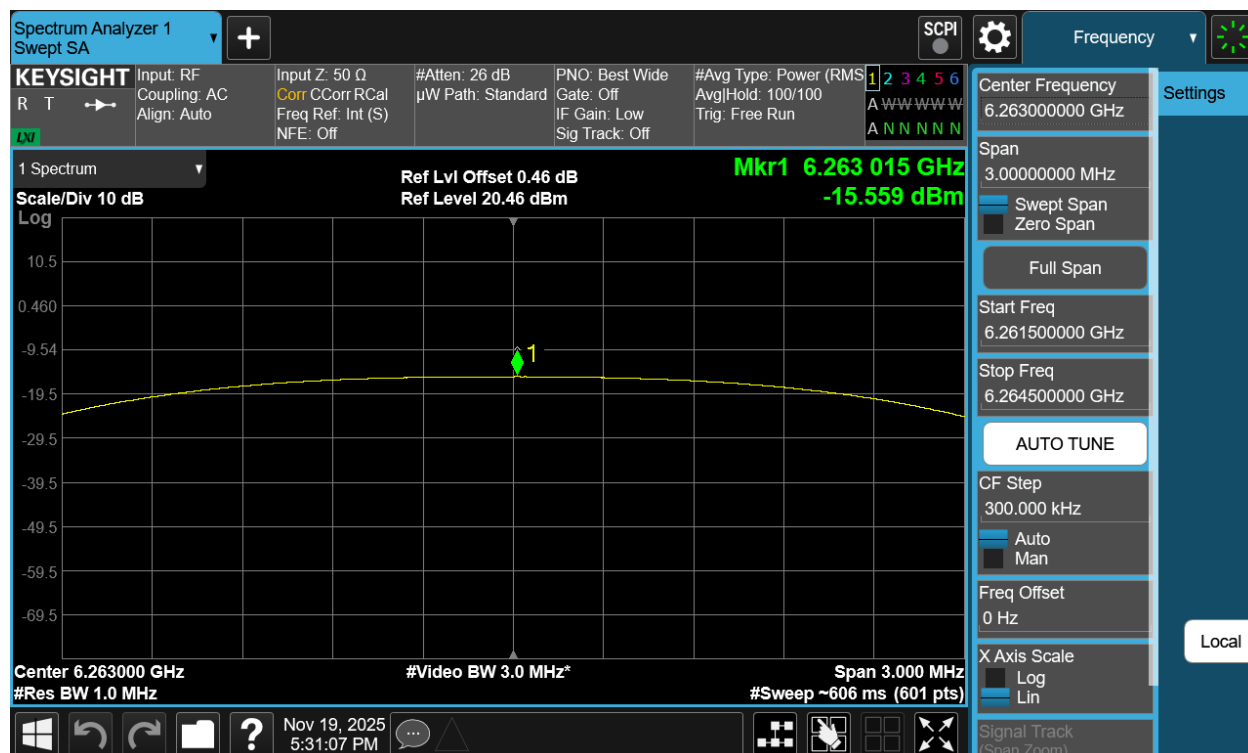
Plot 7-220. PSD Tx BF Diversity Antenna 5T (NB UNII HDT6, iPA – 6263MHz)
