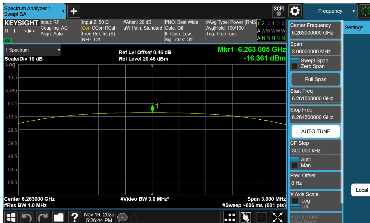
Plot 7-218. PSD Tx BF Diversity Antenna 5T (NB UNII HDT6, ePA – 6263MHz)
