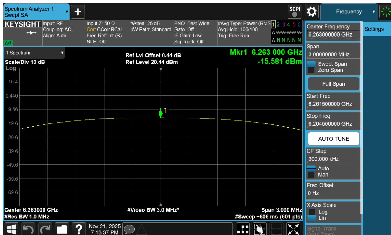
Plot 7-219. PSD Tx BF Diversity Antenna 1b (NB UNII HDT6, ePA – 6263MHz)
