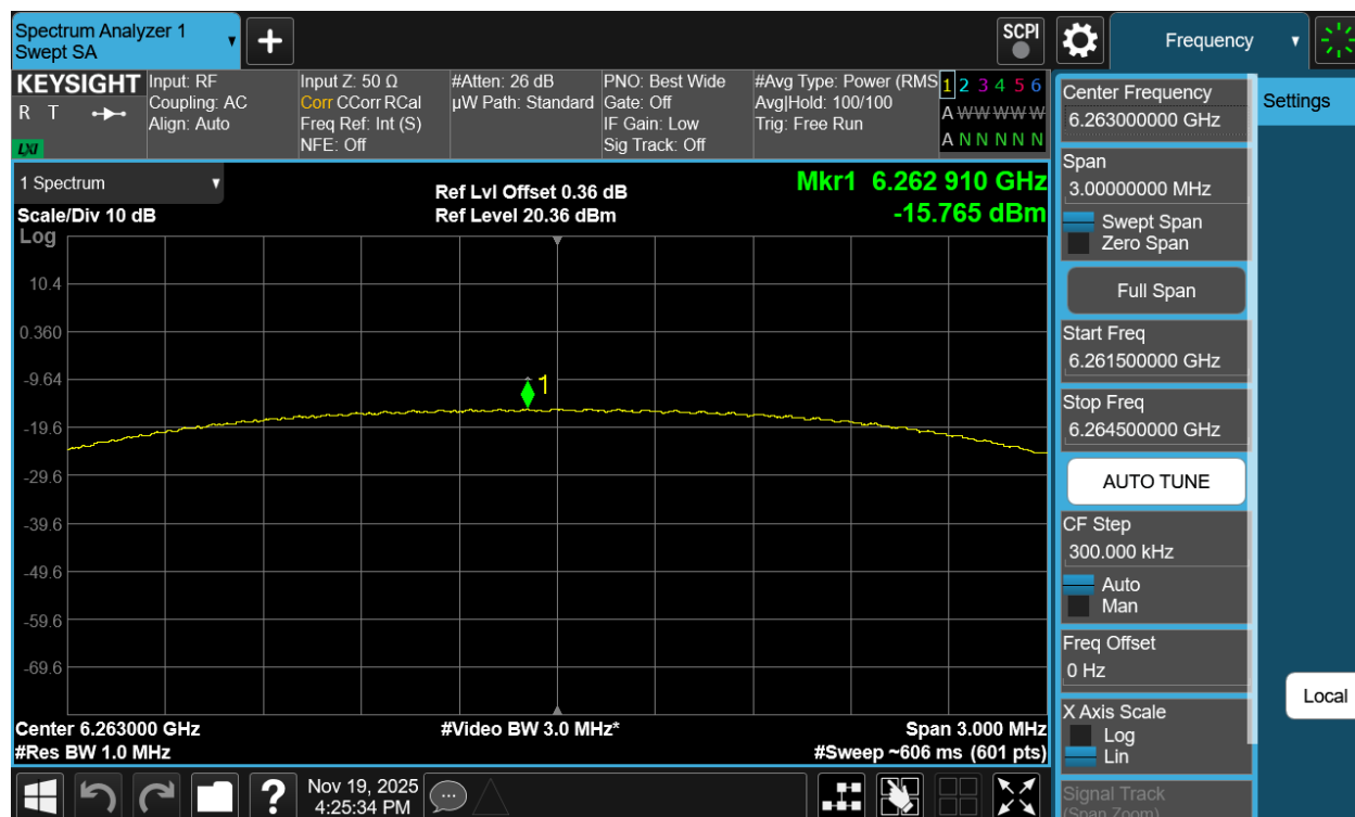
Plot 7-190. PSD TxBF Diversity Antenna 5T (NB UNII HDRPS2, ePA – 6263MHz)
