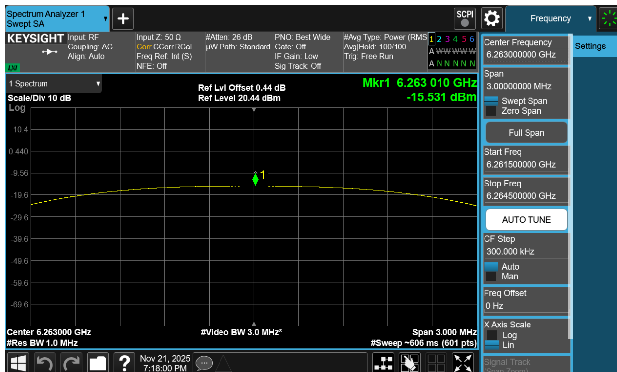
Plot 7-221. PSD Tx BF Diversity Antenna 1b (NB UNII HDT6, iPA – 6263MHz)
