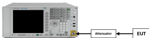
Figure 7-4. Test Instrument & Measurement Setup
