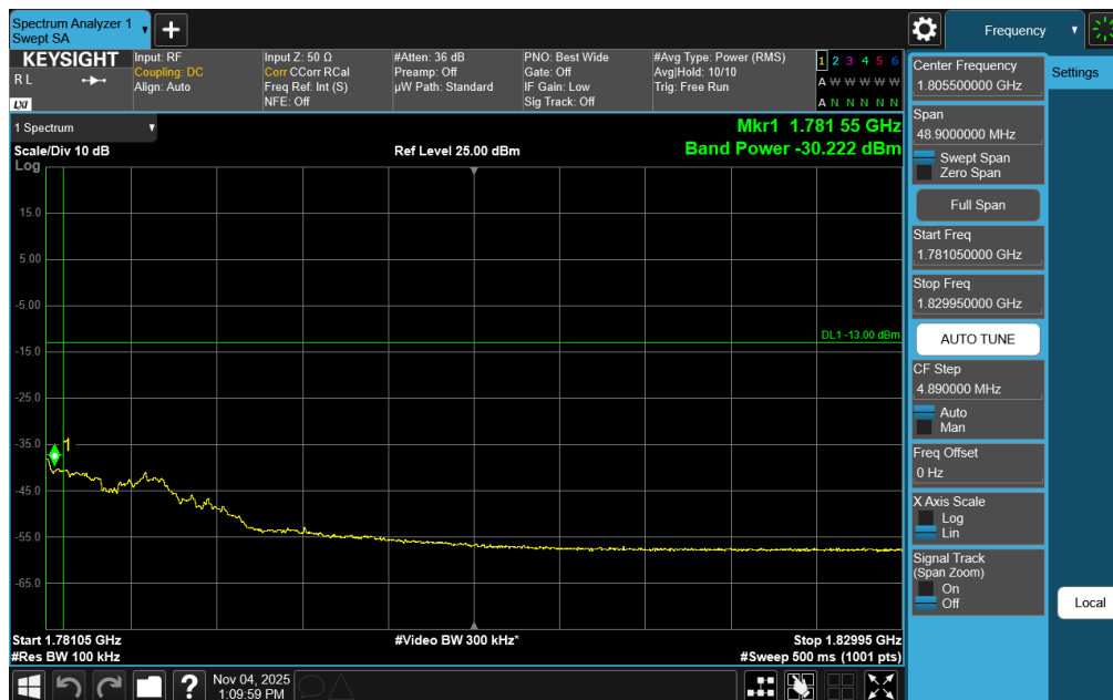
Plot 7-320. Upper Extended Band Edge Plot (NR Band n66 – 5.0MHz DFT-s-OFDM QPSK - Full RB)
