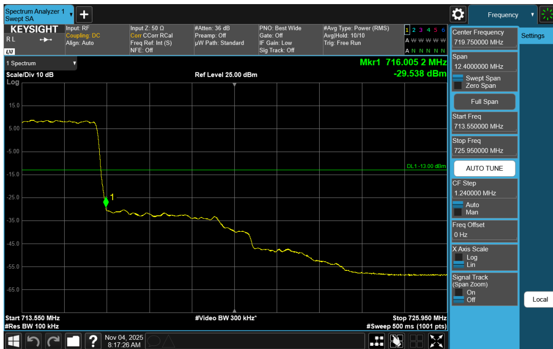
Plot 7-374. Upper Band Edge Plot (NR Band n12 – 5.0MHz DFT-s-OFDM QPSK- Full RB)
