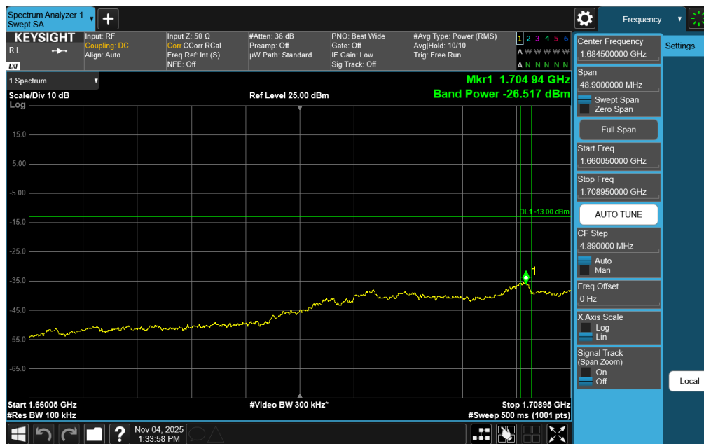
Plot 7-338. Lower Extended Band Edge Plot (NR Band n66 – 30.0MHz DFT-s-OFDM QPSK - Full RB)
