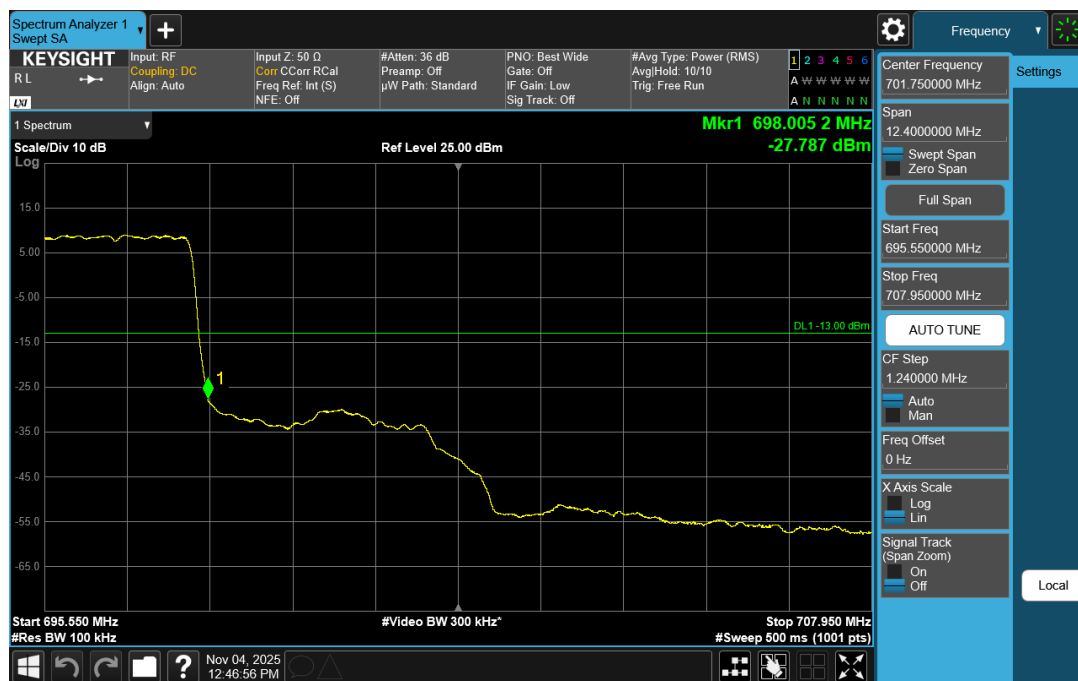
Plot 7-366. Upper Band Edge Plot (NR Band n71 – 5.0MHz DFT-s-OFDM \pi/2 BPSK - Full RB)
