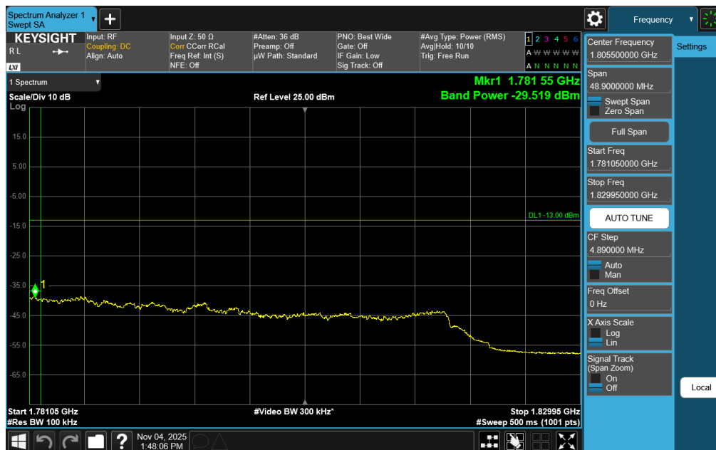
Plot 7-348. Upper Extended Band Edge Plot (NR Band n66 – 40.0MHz DFT-s-OFDM QPSK - Full RB)
