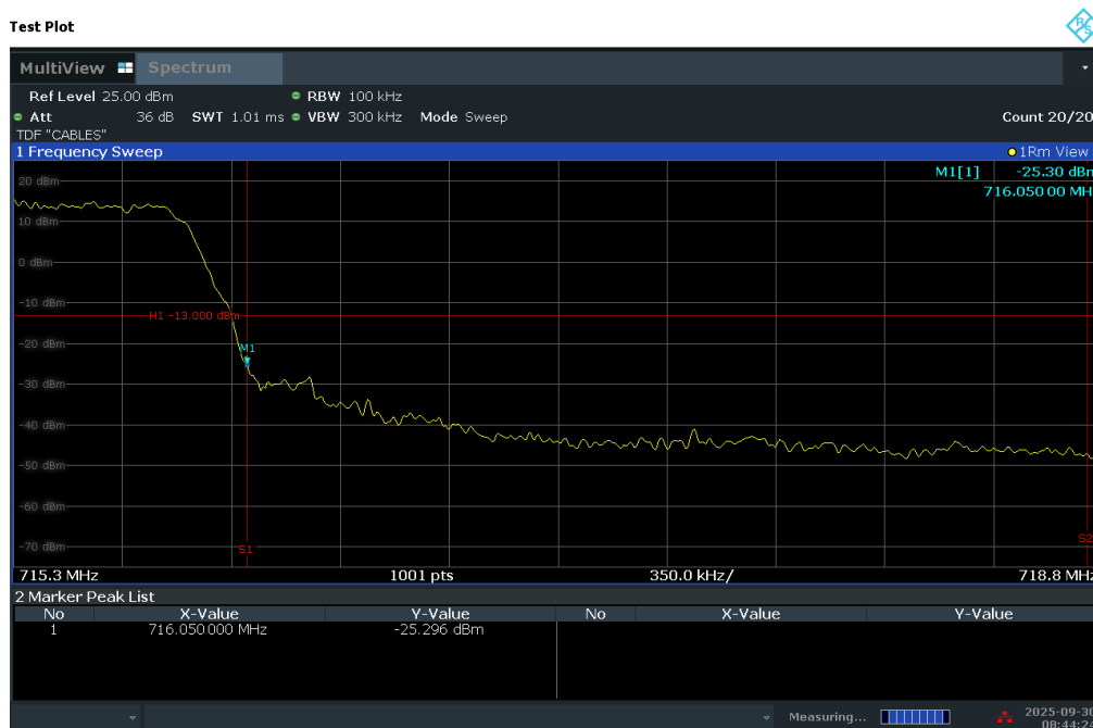
Plot 7-298. Upper Band Edge Plot (LTE Band 12 – 1.4MHz QPSK – Full RB)
