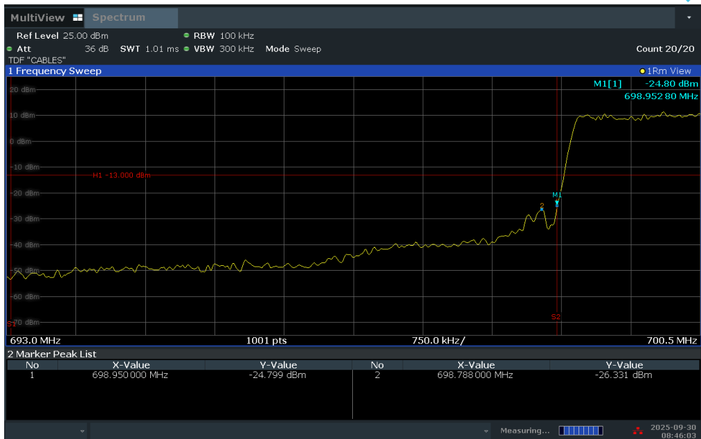
Plot 7-299. Lower Band Edge Plot (LTE Band 12 - 3MHz QPSK – Full RB)
