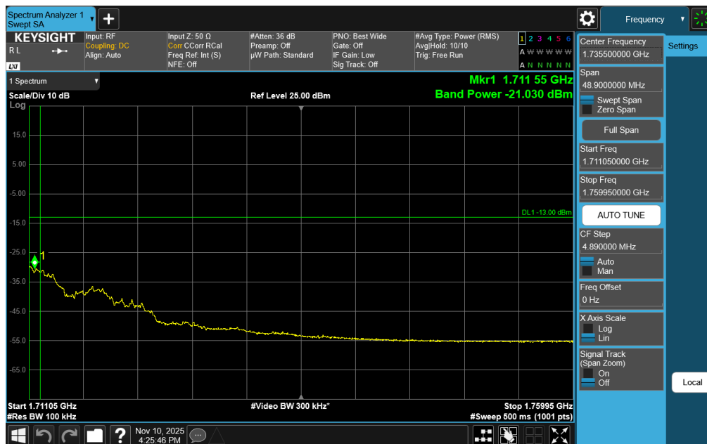
Plot 7-356. Upper Extended Band Edge Plot (NR Band n70 – 5.0MHz DFT-s-OFDM QPSK - Full RB)
