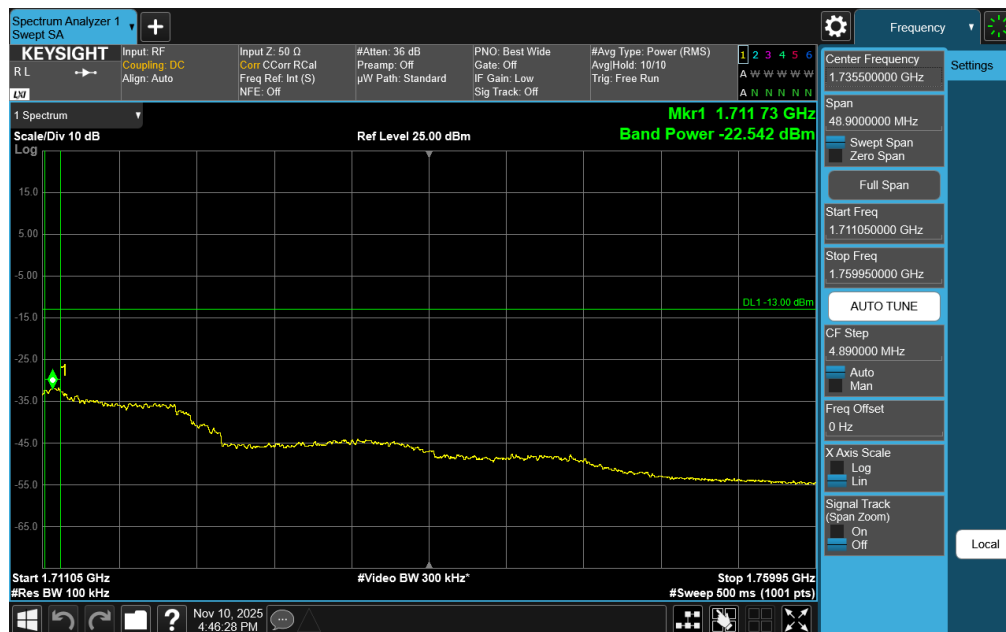
Plot 7-364. Upper Extended Band Edge Plot (NR Band n70 – 15.0MHz DFT-s-OFDM QPSK - Full RB)
