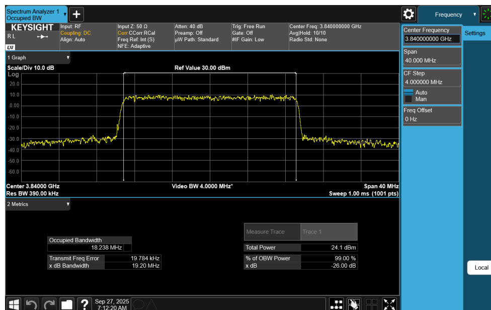
Plot 7-74. Occupied Bandwidth Plot (NR Band n77 C-Band - 20MHz CP-OFDM 64-QAM - Full RB)
