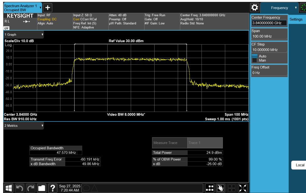
Plot 7-93. Occupied Bandwidth Plot (NR Band n77 C-Band - 50MHz CP-OFDM 16-QAM - Full RB)
