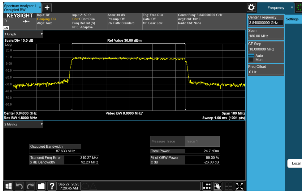
Plot 7-113. Occupied Bandwidth Plot (NR Band n77 C-Band - 90MHz CP-OFDM 16-QAM - Full RB)
