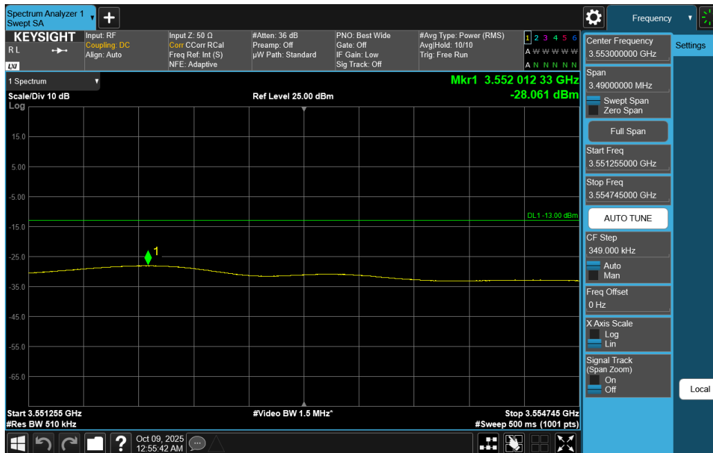
Plot 7-149. Extended Upper Band Edge Plot (NR Band n77 DoD-Band - 15MHz DFT-s-OFDM QPSK – Full RB)
