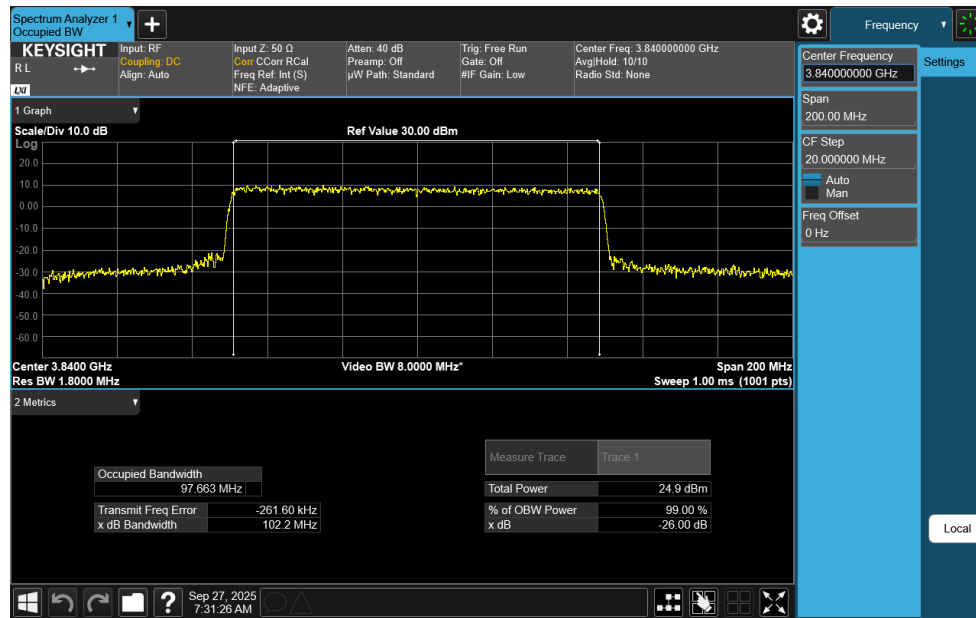
Plot 7-117. Occupied Bandwidth Plot (NR Band n77 C-Band - 100MHz CP-OFDM QPSK - Full RB)
