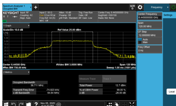
Plot 7-6 26dB BW & 99% OBW Antenna 5T (40MHz BW 802.11be(SU) - Ch.99)
