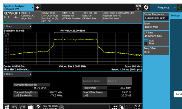
Plot 7-32 26dB BW & 99% OBW Antenna 3b (160MHz BW 802.11be(SU) - Ch.207)
