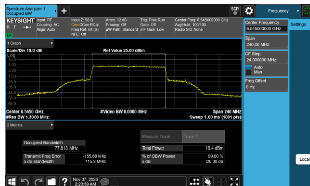
Plot 7-43 26dB BW & 99% OBW Antenna 1b (80MHz BW 802.11be(SU) - Ch.119)
