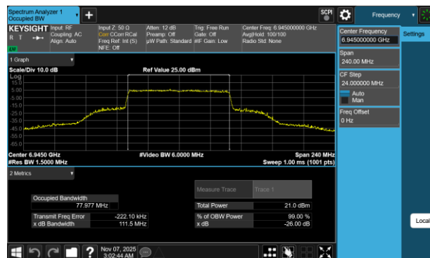
Plot 7-47 26dB BW & 99% OBW Antenna 1b (80MHz BW 802.11be(SU) - Ch.199)
