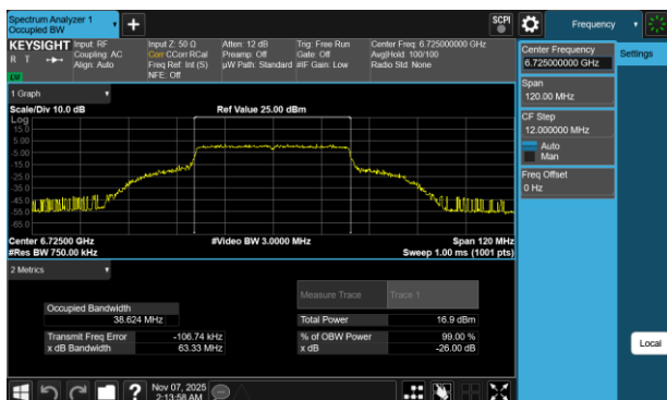
Plot 7-42 26dB BW & 99% OBW Antenna 1b (40MHz BW 802.11be(SU) - Ch.155)
