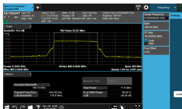
Plot 7-8 26dB BW & 99% OBW Antenna 5T (160MHz BW 802.11be(SU) - Ch.111)
