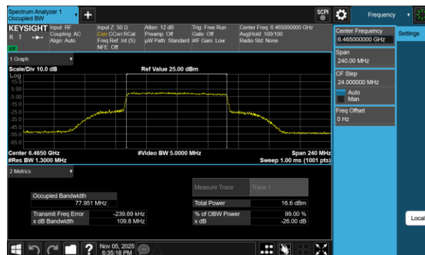
Plot 7-7 26dB BW & 99% OBW Antenna 5T (80MHz BW 802.11be(SU) - Ch.103)
