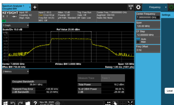
Plot 7-30 26dB BW & 99% OBW Antenna 3b (40MHz BW 802.11be(SU) - Ch.227)
