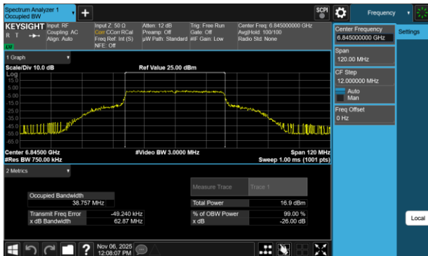
Plot 7-26 26dB BW & 99% OBW Antenna 3b (40MHz BW 802.11be(SU) - Ch.179)
