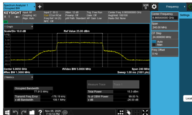
Plot 7-11 26dB BW & 99% OBW Antenna 5T (80MHz BW 802.11be(SU) - Ch.183)
