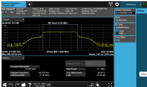
Plot 7-33 26dB BW & 99% OBW Antenna 1b (20MHz BW 802.11be(SU) - Ch.93)
