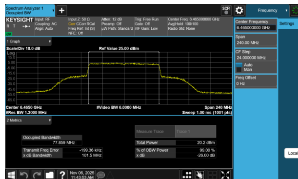
Plot 7-23 26dB BW & 99% OBW Antenna 3b (80MHz BW 802.11be(SU) - Ch.103)
