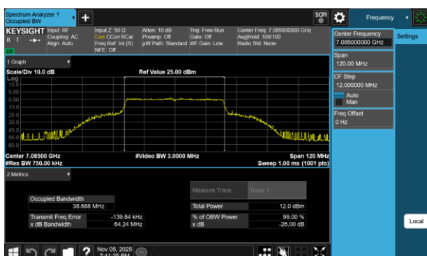
Plot 7-14 26dB BW & 99% OBW Antenna 5T (40MHz BW 802.11be(SU) - Ch.227)
