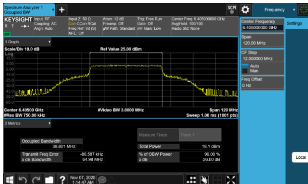
Plot 7-34 26dB BW & 99% OBW Antenna 1b (40MHz BW 802.11be(SU) - Ch.91)
