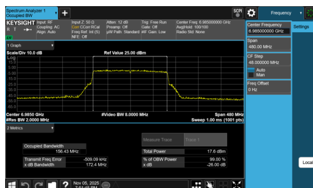
Plot 7-16 26dB BW & 99% OBW Antenna 5T (160MHz BW 802.11be(SU) - Ch.207)
