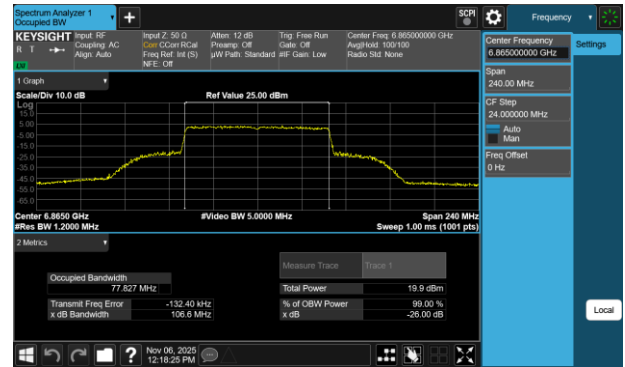
Plot 7-27 26dB BW & 99% OBW Antenna 3b (80MHz BW 802.11be(SU) - Ch.183)
