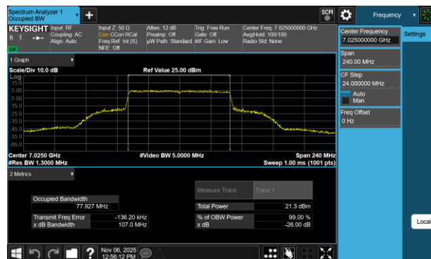
Plot 7-31 26dB BW & 99% OBW Antenna 3b (80MHz BW 802.11be(SU) - Ch.215)
