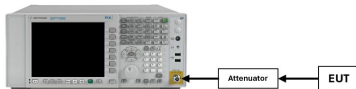
Figure 7-1. Test Instrument & Measurement Setup
