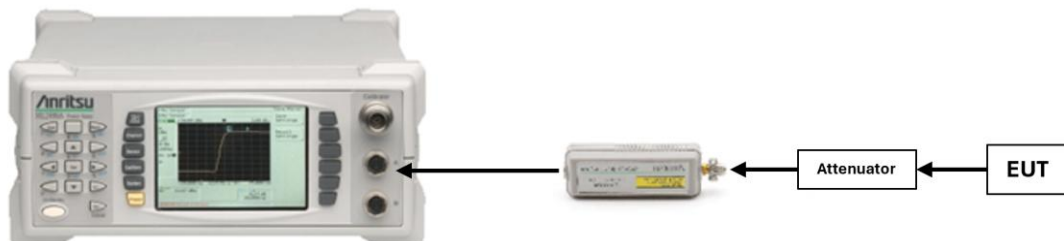
Figure 7-2. Test Instrument & Measurement Setup
