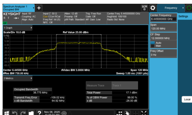
Plot 7-22 26dB BW & 99% OBW Antenna 3b (40MHz BW 802.11be(SU) - Ch.99)
