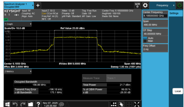
Plot 7-36 26dB BW & 99% OBW Antenna 1b (160MHz BW 802.11be(SU) - Ch.47)
