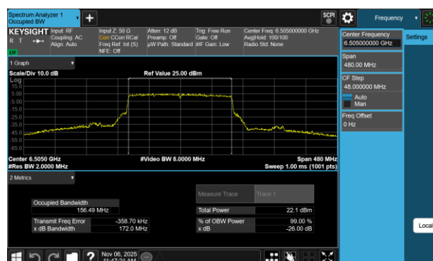
Plot 7-24 26dB BW & 99% OBW Antenna 3b (160MHz BW 802.11be(SU) - Ch.111)
