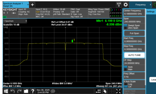
Plot 7-68 PSD Antenna 3b (160MHz BW 802.11be(SU) - Ch.47)
