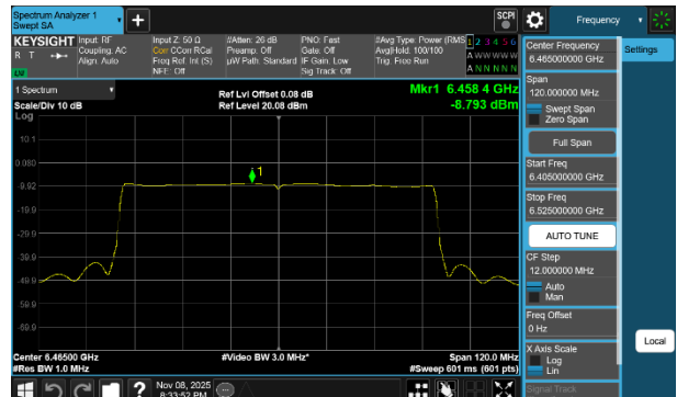
Plot 7-207 PSD SDM Primary Antenna 3b (80MHz BW 802.11be(SU) - Ch.103)
