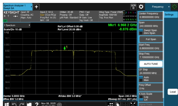
Plot 7-224 PSD SDM Primary Antenna 3b (160MHz BW 802.11be(SU) - Ch.207)
