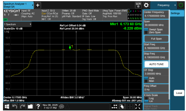
Plot 7-197 PSD SDM Primary Antenna 3b (20MHz BW 802.11be(SU) - Ch.45)
