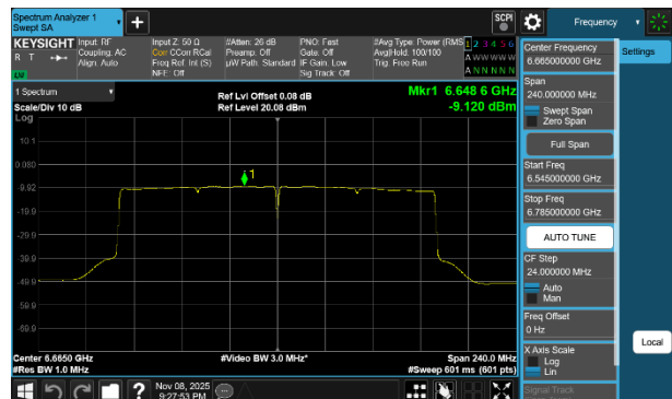
Plot 7-216 PSD SDM Primary Antenna 3b (160MHz BW 802.11be(SU) - Ch.143)
