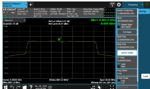
Plot 7-214 PSD SDM Primary Antenna 3b (40MHz BW 802.11be(SU) - Ch.123)
