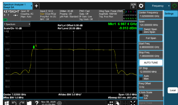
Plot 7-223 PSD SDM Primary Antenna 3b (80MHz BW 802.11be(SU) - Ch.215)
