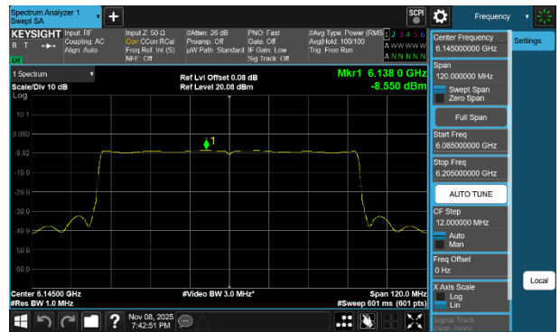
Plot 7-199 PSD SDM Primary Antenna 3b (80MHz BW 802.11be(SU) - Ch.39)
