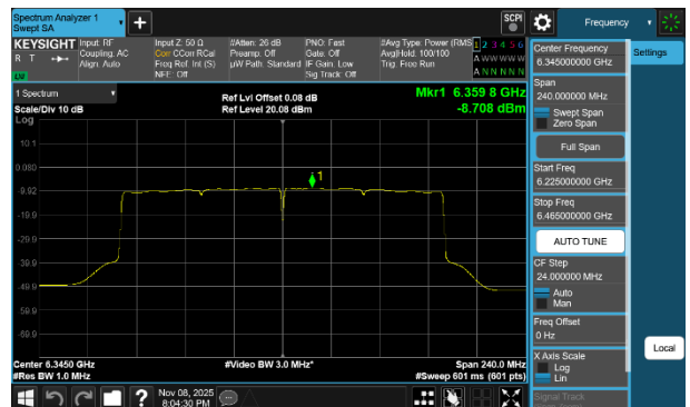
Plot 7-200 PSD SDM Primary Antenna 3b (160MHz BW 802.11be(SU) - Ch.79)
