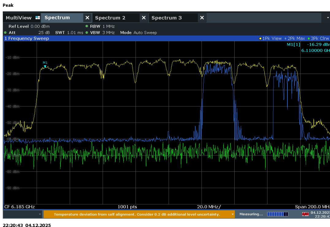
Plot 7-321. 160MHz Bandwidth, AWGN Signal Injected – 6430Mhz
