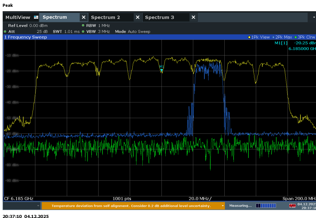
Plot 7-322. 160MHz Bandwidth, AWGN Signal Injected – 6505MHz
