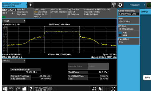
Plot 7-185 26dB BW & 99% OBW Antenna 1b (40MHz BW 802.11be(RU) RU484 Index65 - Ch.179)
