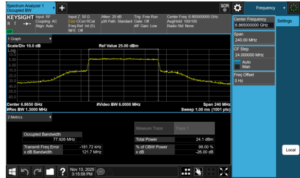
Plot 7-219 26dB BW & 99% OBW Antenna 1b (80MHz BW 802.11be(RU) RU996 Index67 - Ch.183)
