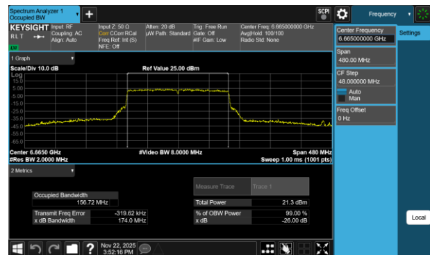
Plot 7-187 26dB BW & 99% OBW Antenna 1b (160MHz BW 802.11be(RU) RU996X2 Index68 - Ch.143)
