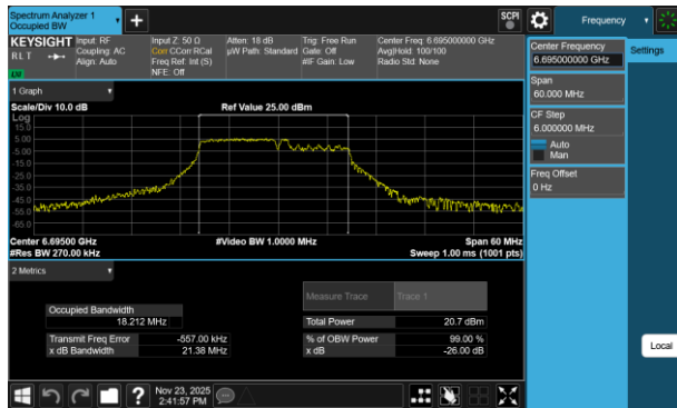
Plot 7-181 26dB BW & 99% OBW Antenna 1b (20MHz BW 802.11be(RU) RU106+26 Index82 - Ch.149)
