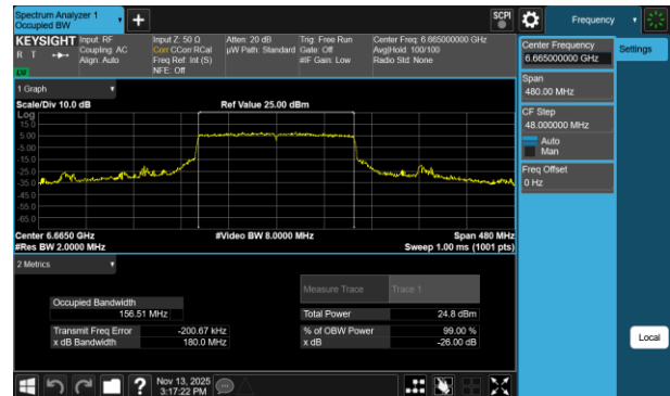
Plot 7-220 26dB BW & 99% OBW Antenna 1b (160MHz BW 802.11be(RU) RU996X2 Index68 - Ch.143)
