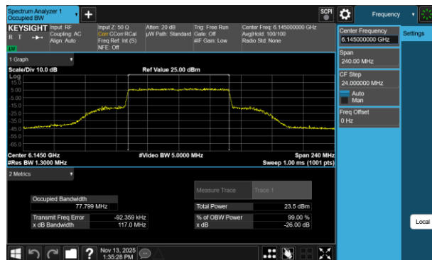
Plot 7-197 26dB BW & 99% OBW Antenna 1b (80MHz BW 802.11be(RU) RU996 Index67 - Ch.39)
