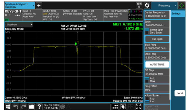
Plot 7-242 PSD Antenna 5T (160MHz BW 802.11be(RU) RU996X2 Index68 - Ch.47)
