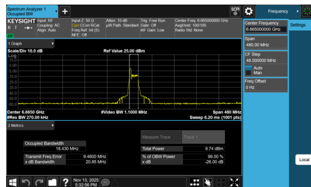
Plot 7-213 26dB BW & 99% OBW Antenna 1b (160MHz BW 802.11be(RU) RU26 Index0 - Ch.143)
