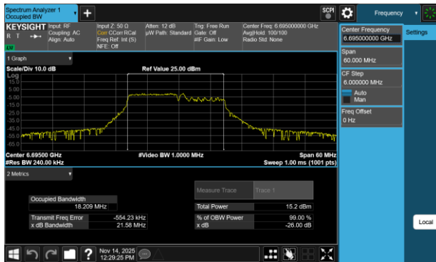
Plot 7-214 26dB BW & 99% OBW Antenna 1b (20MHz BW 802.11be(RU) RU106+26 Index82 - Ch.149)
