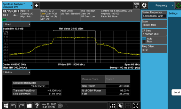
Plot 7-184 26dB BW & 99% OBW Antenna 1b (20MHz BW 802.11be(RU) RU242 Index61 - Ch.149)
