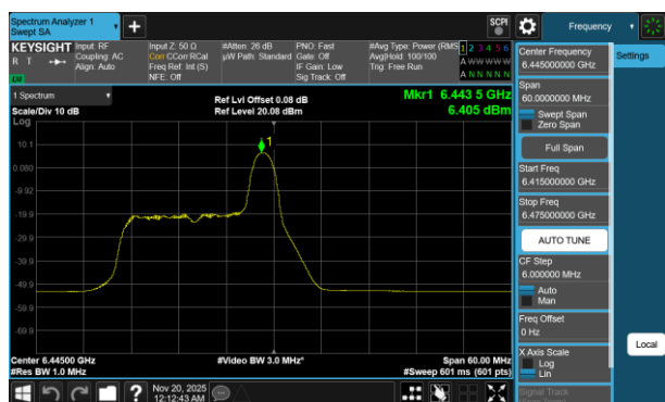
Plot 7-244 PSD Antenna 5T (40MHz BW 802.11be(RU) RU26 Index8 - Ch.99)
