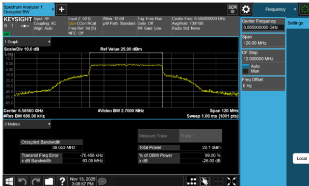
Plot 7-218 26dB BW & 99% OBW Antenna 1b (40MHz BW 802.11be(RU) RU484 Index65 - Ch.123)
