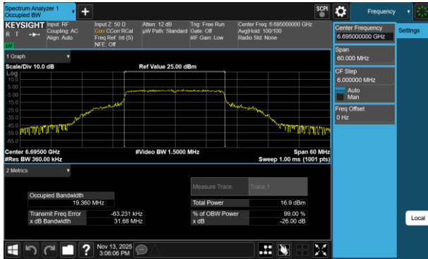
Plot 7-217 26dB BW & 99% OBW Antenna 1b (20MHz BW 802.11be(RU) RU242 Index61 - Ch.149)
