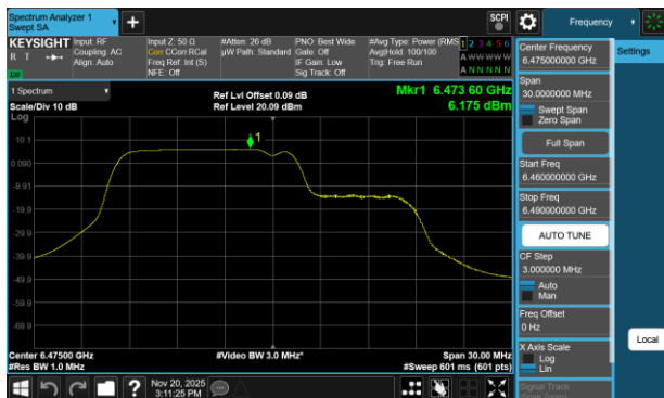
Plot 7-247 PSD Antenna 5T (20MHz BW 802.11be(RU) RU106+26 Index82 - Ch.105)
