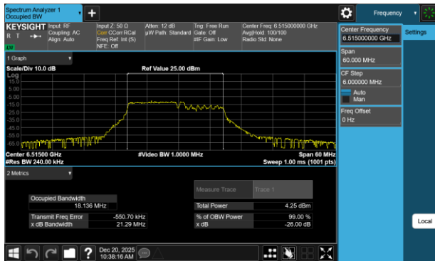
Plot 7-203 26dB BW & 99% OBW Antenna 1b (20MHz BW 802.11be(RU) RU106+26 Index82 - Ch.113)
