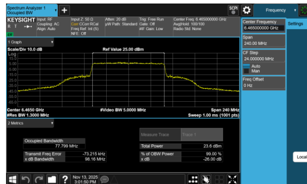
Plot 7-208 26dB BW & 99% OBW Antenna 1b (80MHz BW 802.11be(RU) RU996 Index67 - Ch.103)
