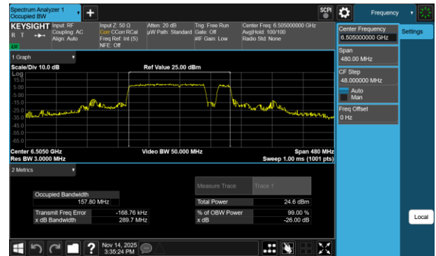
Plot 7-205 26dB BW & 99% OBW Antenna 1b (160MHz BW 802.11be(RU) RU996+484+242 Index98 - Ch.111)
