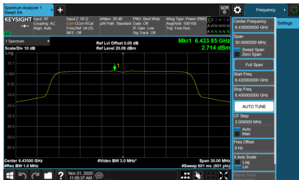
Plot 7-327 PSD Antenna 3b (20MHz BW 802.11be(RU) RU242 Index61 - Ch.97)
