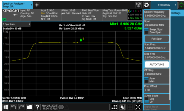
Plot 7-316 PSD Antenna 3b (20MHz BW 802.11be(RU) RU242 Index61 - Ch.1)
