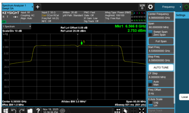
Plot 7-262 PSD Antenna 5T (40MHz BW 802.11be(RU) RU484 Index65 - Ch.123)
