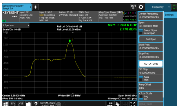
Plot 7-332 PSD Antenna 3b (40MHz BW 802.11be(RU) RU26 Index8 - Ch.123)
