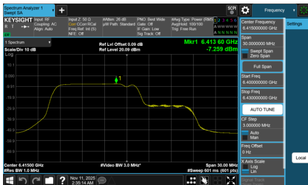
Plot 7-269 PSD Antenna 5T (20MHz BW 802.11be(RU) RU106+26 Index82 - Ch.93)
