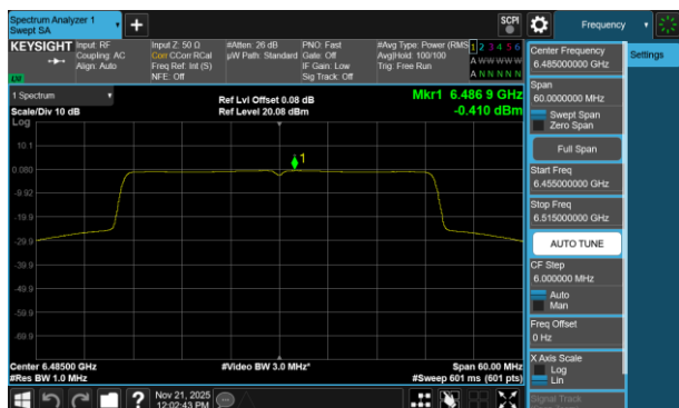
Plot 7-328 PSD Antenna 3b (40MHz BW 802.11be(RU) RU484 Index65 - Ch.107)
