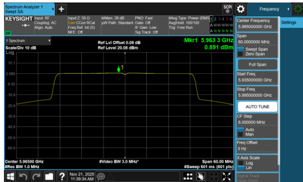
Plot 7-317 PSD Antenna 3b (40MHz BW 802.11be(RU) RU484 Index65 - Ch.3)
