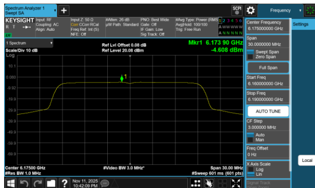
Plot 7-349 PSD Antenna 3b (20MHz BW 802.11be(RU) RU242 Index61 - Ch.45)
