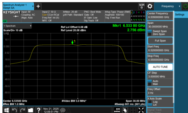
Plot 7-338 PSD Antenna 3b (20MHz BW 802.11be(RU) RU242 Index61 - Ch.117)
