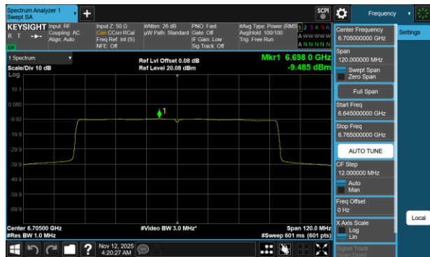
Plot 7-593 PSD CDD Primary Antenna 3b (80MHz BW 802.11be(RU) RU996 Index67 - Ch.151)
