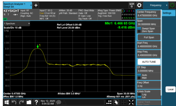
Plot 7-555 PSD CDD Primary Antenna 3b (20MHz BW 802.11be(RU) RU26 Index0 - Ch.105)
