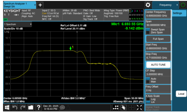
Plot 7-584 PSD CDD Primary Antenna 3b (20MHz BW 802.11be(RU) RU106+26 Index82 - Ch.149)
