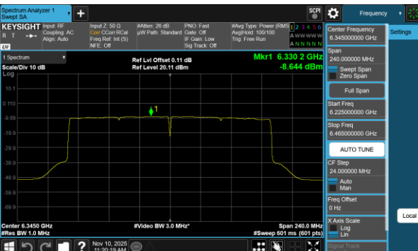
Plot 7-546 PSD CDD Primary Antenna 5T (160MHz BW 802.11be(RU) RU996X2 Index68 - Ch.79)
