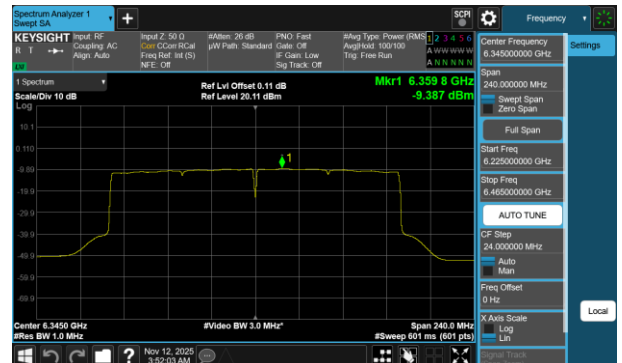
Plot 7-550 PSD CDD Primary Antenna 3b (160MHz BW 802.11be(RU) RU996X2 Index68 - Ch.79)
