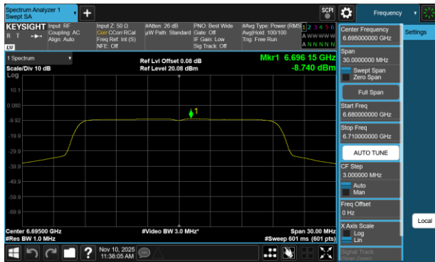
Plot 7-587 PSD CDD Primary Antenna 5T (20MHz BW 802.11be(RU) RU242 Index61 - Ch.149)
