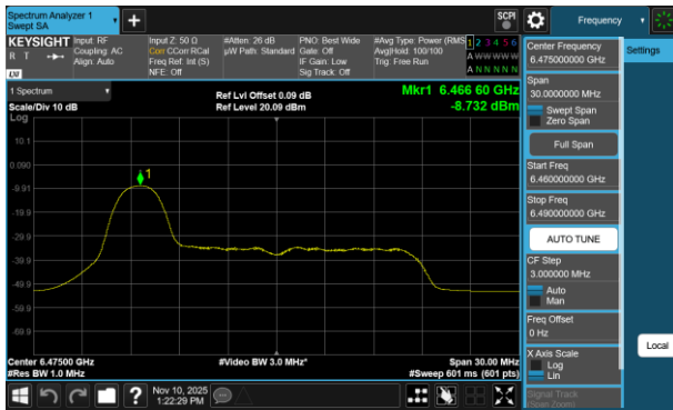
Plot 7-551 PSD CDD Primary Antenna 5T (20MHz BW 802.11be(RU) RU26 Index0 - Ch.105)
