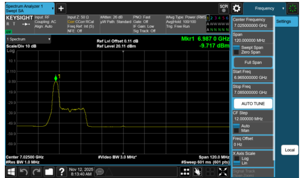
Plot 7-601 PSD CDD Primary Antenna 3b (80MHz BW 802.11be(RU) RU26 Index0 - Ch.215)
