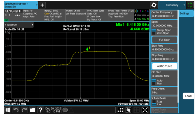
Plot 7-540 PSD CDD Primary Antenna 3b (20MHz BW 802.11be(RU) RU106+26 Index83 - Ch.93)
