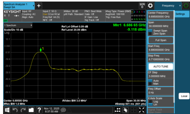
Plot 7-577 PSD CDD Primary Antenna 3b (20MHz BW 802.11be(RU) RU26 Index0 - Ch.149)
