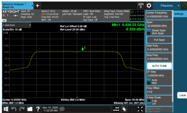
Plot 7-565 PSD CDD Primary Antenna 5T (20MHz BW 802.11be(RU) RU242 Index61 - Ch.97)
