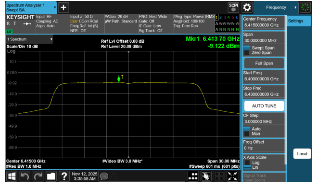
Plot 7-547 PSD CDD Primary Antenna 3b (20MHz BW 802.11be(RU) RU242 Index61 - Ch.93)
