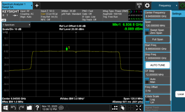
Plot 7-611 PSD CDD Primary Antenna 5T (80MHz BW 802.11be(RU) RU996 Index67 - Ch.199)
