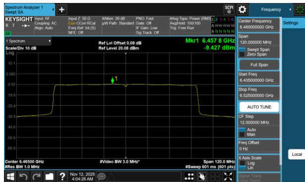
Plot 7-571 PSD CDD Primary Antenna 3b (80MHz BW 802.11be(RU) RU996 Index67 - Ch.103)
