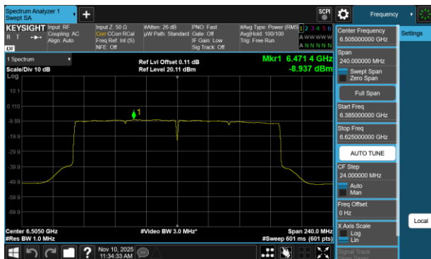
Plot 7-568 PSD CDD Primary Antenna 5T (160MHz BW 802.11be(RU) RU996X2 Index68 - Ch.111)
