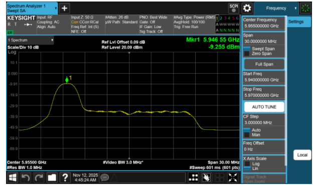
Plot 7-533 PSD CDD Primary Antenna 3b (20MHz BW 802.11be(RU) RU26 Index0 - Ch.1)
