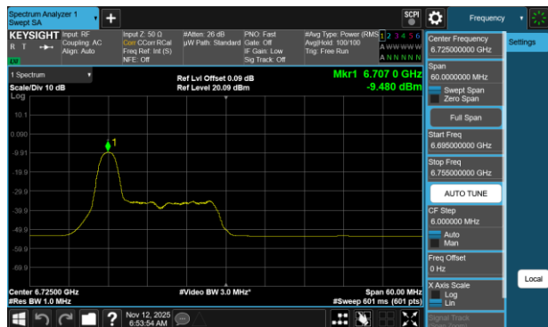
Plot 7-578 PSD CDD Primary Antenna 3b (40MHz BW 802.11be(RU) RU26 Index0 - Ch.155)
