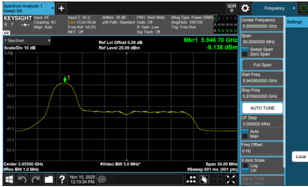
Plot 7-529 PSD CDD Primary Antenna 5T (20MHz BW 802.11be(RU) RU26 Index0 - Ch.1)
