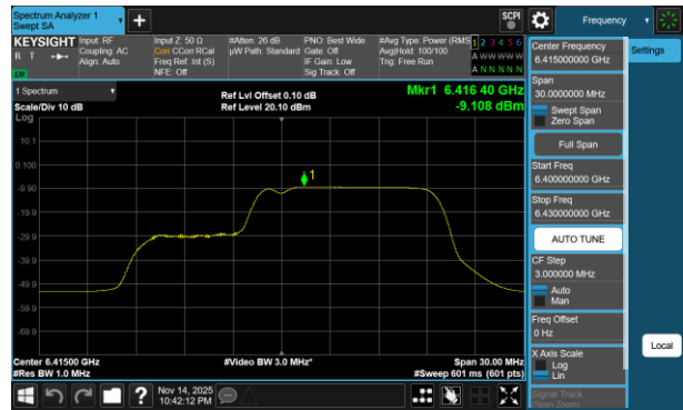
Plot 7-694 PSD CDD Diversity Antenna 1b (20MHz BW 802.11be(RU) RU106+26 Index83 - Ch.93)
