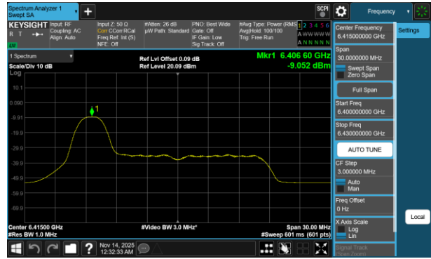
Plot 7-687 PSD CDD Diversity Antenna 1b (20MHz BW 802.11be(RU) RU26 Index0 - Ch.93)
