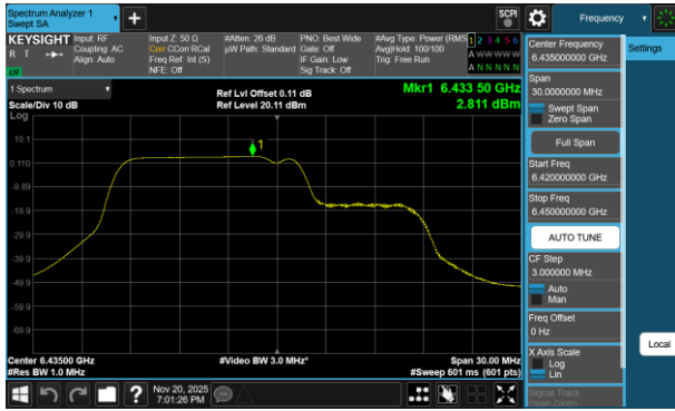
Plot 7-647 PSD CDD Diversity Antenna 5T (20MHz BW 802.11be(RU) RU106+26 Index82 - Ch.97)
