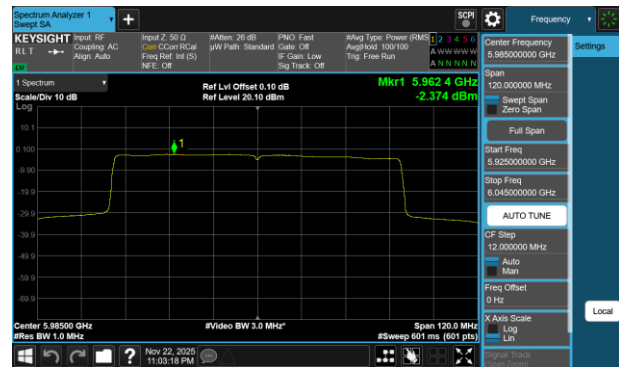
Plot 7-637 PSD CDD Diversity Antenna 1b (80MHz BW 802.11be(RU) RU996 Index67 - Ch.7)
