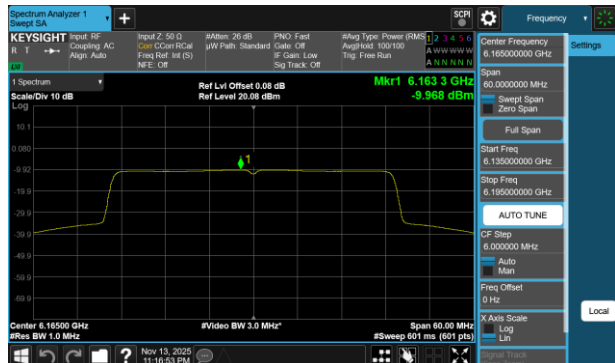
Plot 7-702 PSD CDD Diversity Antenna 1b (40MHz BW 802.11be(RU) RU484 Index65 - Ch.43)
