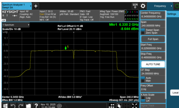
Plot 7-700 PSD CDD Diversity Antenna 5T (160MHz BW 802.11be(RU) RU996X2 Index68 - Ch.79)
