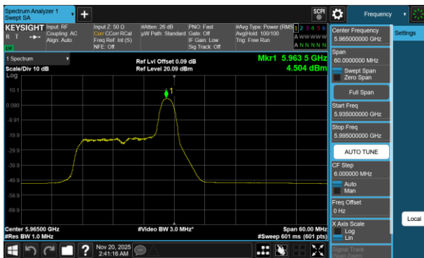
Plot 7-618 PSD CDD Diversity Antenna 5T (40MHz BW 802.11be(RU) RU26 Index8 - Ch.3)
