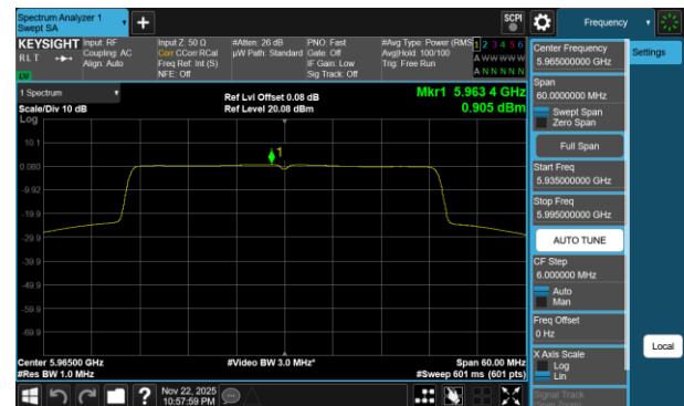
Plot 7-636 PSD CDD Diversity Antenna 1b (40MHz BW 802.11be(RU) RU484 Index65 - Ch.3)
