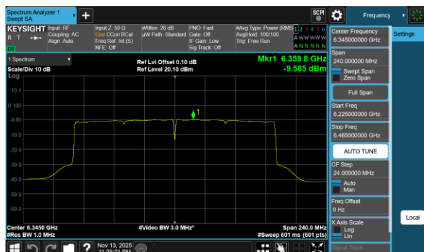
Plot 7-704 PSD CDD Diversity Antenna 1b (160MHz BW 802.11be(RU) RU996X2 Index68 - Ch.79)
