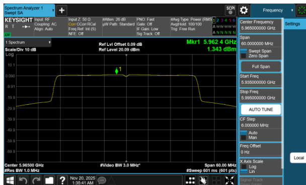
Plot 7-632 PSD CDD Diversity Antenna 5T (40MHz BW 802.11be(RU) RU484 Index65 - Ch.3)
