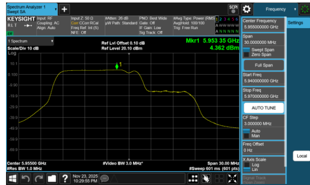
Plot 7-628 PSD CDD Diversity Antenna 1b (20MHz BW 802.11be(RU) RU106+26 Index82 - Ch.1)
