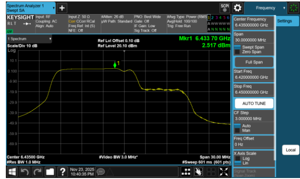
Plot 7-650 PSD CDD Diversity Antenna 1b (20MHz BW 802.11be(RU) RU106+26 Index82 - Ch.97)
