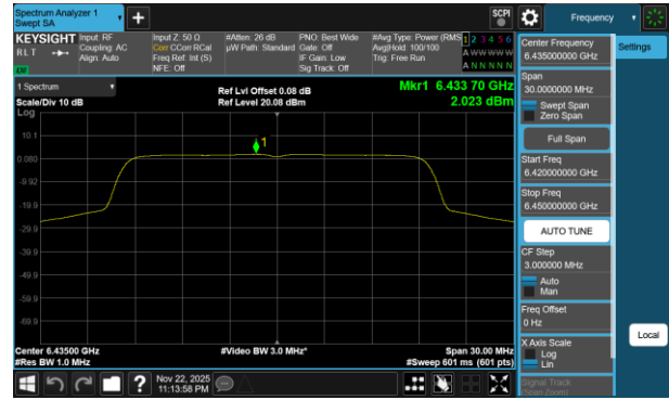
Plot 7-657 PSD CDD Diversity Antenna 1b (20MHz BW 802.11be(RU) RU242 Index61 - Ch.97)
