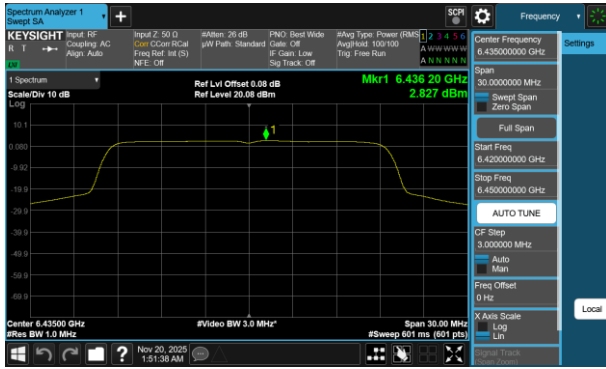
Plot 7-653 PSD CDD Diversity Antenna 5T (20MHz BW 802.11be(RU) RU242 Index61 - Ch.97)
