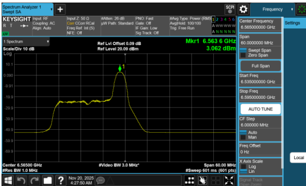
Plot 7-662 PSD CDD Diversity Antenna 5T (40MHz BW 802.11be(RU) RU26 Index8 - Ch.123)
