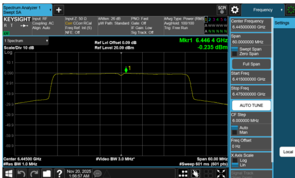
Plot 7-654 PSD CDD Diversity Antenna 5T (40MHz BW 802.11be(RU) RU484 Index65 - Ch.99)
