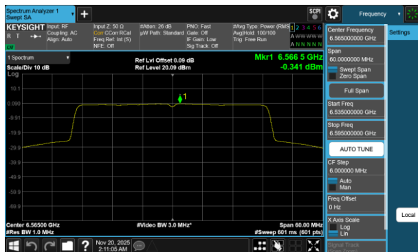
Plot 7-676 PSD CDD Diversity Antenna 5T (40MHz BW 802.11be(RU) RU484 Index65 - Ch.123)
