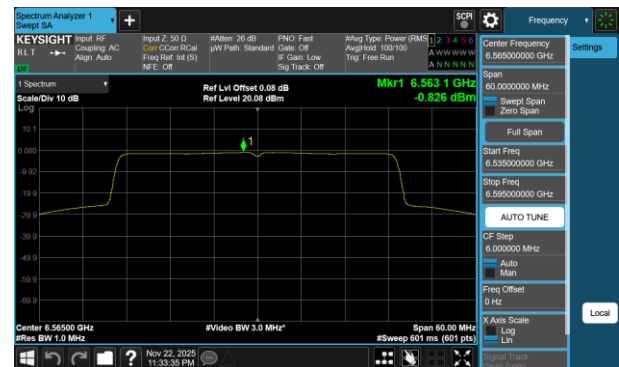
Plot 7-680 PSD CDD Diversity Antenna 1b (40MHz BW 802.11be(RU) RU484 Index65 - Ch.123)
