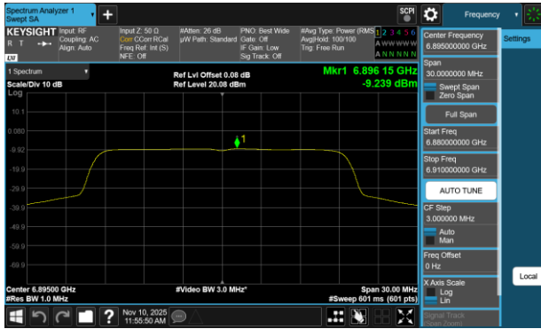
Plot 7-763 PSD CDD Diversity Antenna 5T (20MHz BW 802.11be(RU) RU242 Index61 - Ch.189)
