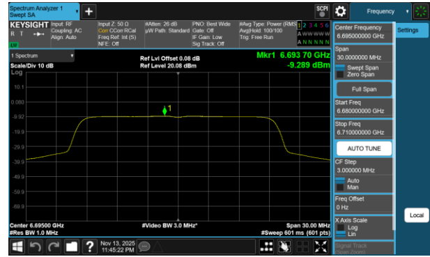
Plot 7-745 PSD CDD Diversity Antenna 1b (20MHz BW 802.11be(RU) RU242 Index61 - Ch.149)
