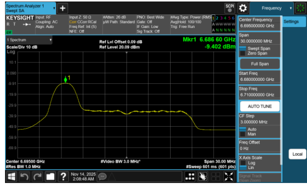
Plot 7-731 PSD CDD Diversity Antenna 1b (20MHz BW 802.11be(RU) RU26 Index0 - Ch.149)
