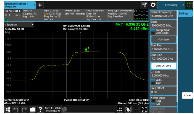
Plot 7-760 PSD CDD Diversity Antenna 1b (20MHz BW 802.11be(RU) RU106+26 Index83 - Ch.209)
