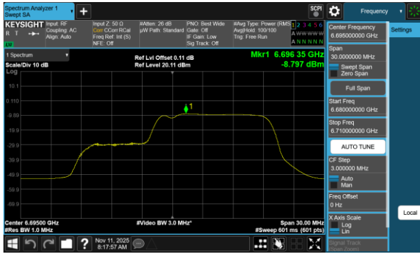
Plot 7-735 PSD CDD Diversity Antenna 5T (20MHz BW 802.11be(RU) RU106+26 Index83 - Ch.149)
