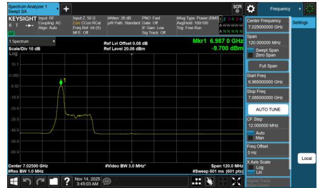
Plot 7-755 PSD CDD Diversity Antenna 1b (80MHz BW 802.11be(RU) RU26 Index0 - Ch.215)
