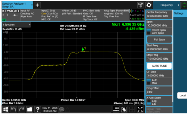
Plot 7-757 PSD CDD Diversity Antenna 5T (20MHz BW 802.11be(RU) RU106+26 Index83 - Ch.209)
