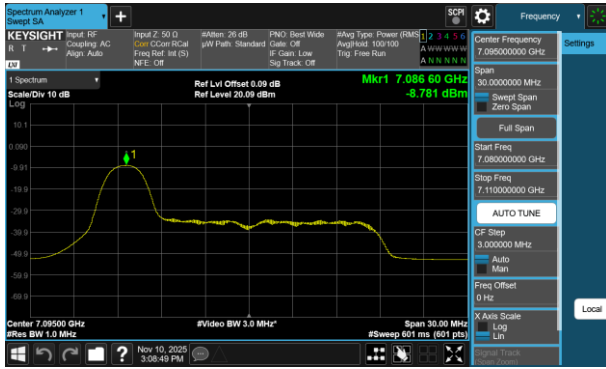
Plot 7-749 PSD CDD Diversity Antenna 5T (20MHz BW 802.11be(RU) RU26 Index0 - Ch.229)
