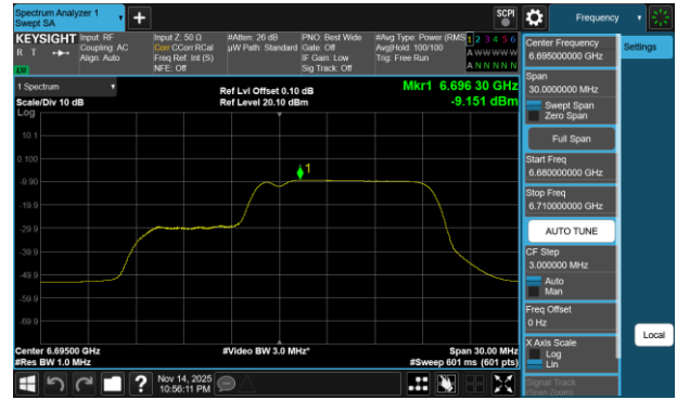
Plot 7-738 PSD CDD Diversity Antenna 1b (20MHz BW 802.11be(RU) RU106+26 Index83 - Ch.149)
