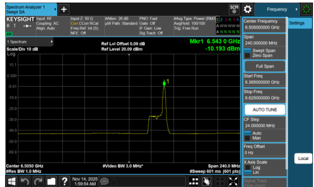
Plot 7-712 PSD CDD Diversity Antenna 1b (160MHz BW 802.11be(RU) RU26 Index17 - Ch.111)
