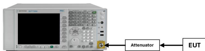
Figure 7-4. Test Instrument & Measurement Setup
