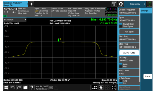
Plot 7-767 PSD CDD Diversity Antenna 1b (20MHz BW 802.11be(RU) RU242 Index61 - Ch.189)
