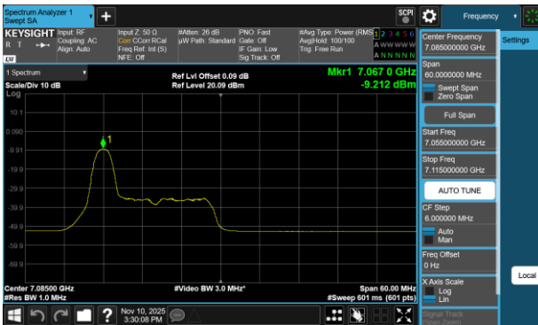
Plot 7-750 PSD CDD Diversity Antenna 5T (40MHz BW 802.11be(RU) RU26 Index0 - Ch.227)
