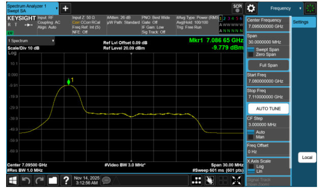
Plot 7-753 PSD CDD Diversity Antenna 1b (20MHz BW 802.11be(RU) RU26 Index0 - Ch.229)
