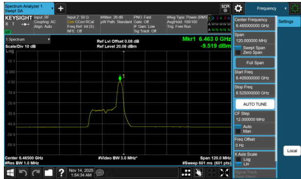
Plot 7-711 PSD CDD Diversity Antenna 1b (80MHz BW 802.11be(RU) RU26 Index17 - Ch.103)
