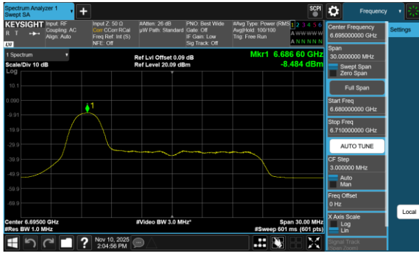
Plot 7-727 PSD CDD Diversity Antenna 5T (20MHz BW 802.11be(RU) RU26 Index0 - Ch.149)
