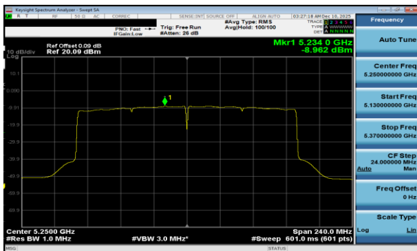
Plot 7-225 PSD CDD Diversity Antenna 1b (160MHz BW 802.11be(RU) RU996X2 Index68 - Ch.50)
