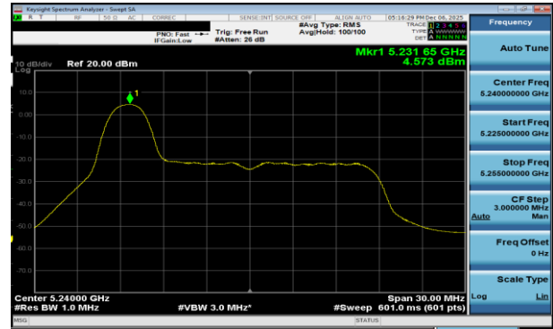
Plot 7-250 PSD SDM Diversity Antenna 5T (20MHz BW 802.11be(RU) RU26 Index0 - Ch.48)
