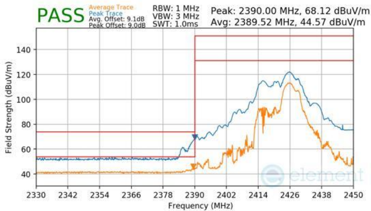
Plot 7-173 Radiated Restricted Lower Band Edge Measurement CDD (Peak & Average – RU52+26)
