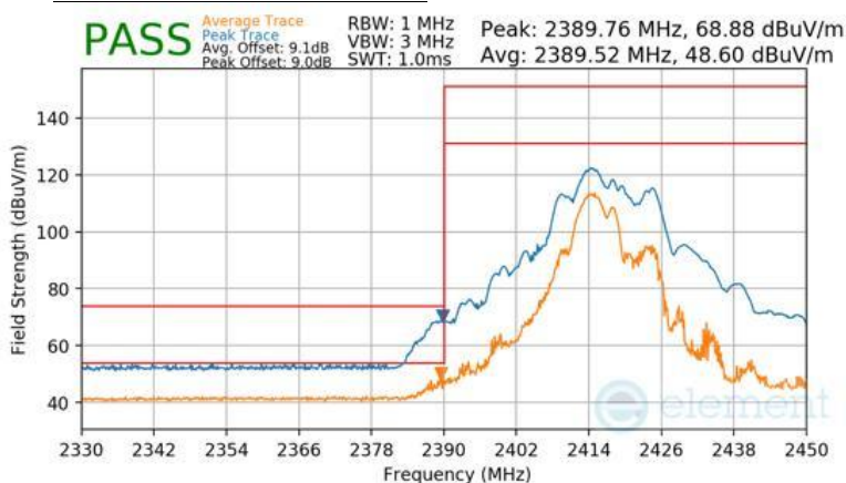
Plot 7-170 Radiated Restricted Lower Band Edge Measurement CDD (Peak & Average – RU52+26)
