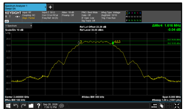
Figure 38 - Core 1 (B) 2440 MHz (CH18) 6 dB Bandwidth
