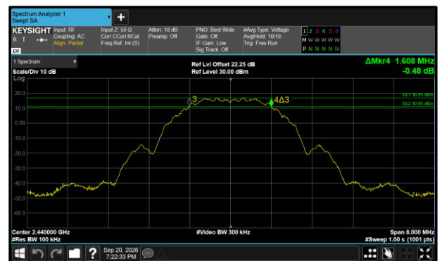
Figure 32 - Core 0 (A) 2440 MHz (CH18) 6 dB Bandwidth
