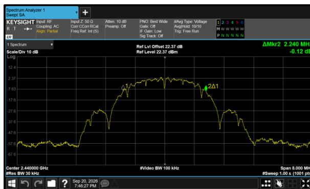
Figure 25 - Core 2 (C) 2440 MHz (CH18) 99% Bandwidth
