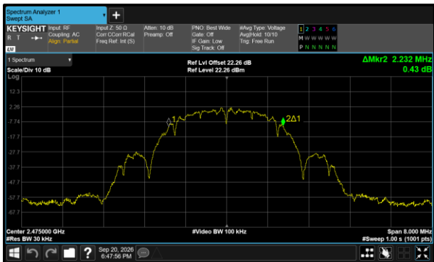
Figure 15 - Core 0 (A) 2475 MHz (CH25) 99% Bandwidth
