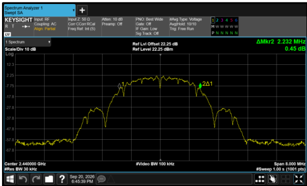
Figure 13 - Core 0 (A) 2440 MHz (CH18) 99% Bandwidth
