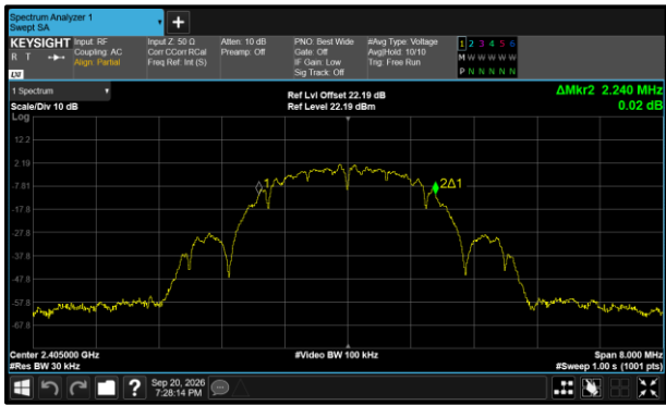
Figure 17 - Core 1 (B) 2405 MHz (CH11) 99% Bandwidth
