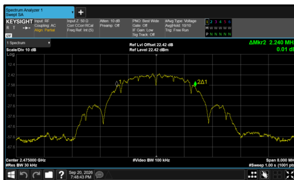
Figure 27 - Core 2 (C) 2475 MHz (CH25) 99% Bandwidth
