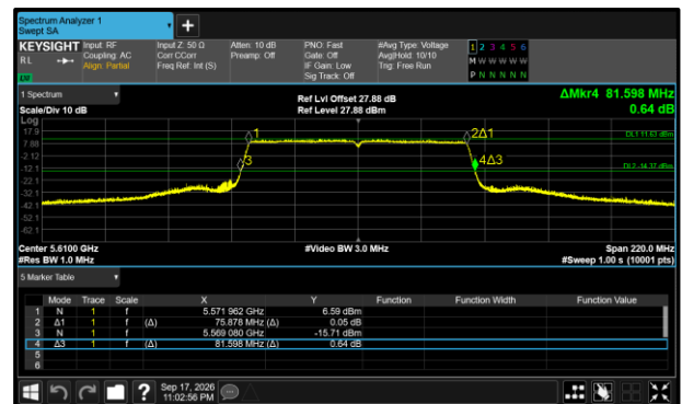
Figure 258 - 802.11ac VHT80 Maximum 26 dB EBW
