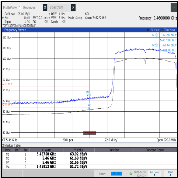
Lower Band Edge / 80 MHz Bandwidth / Restricted Band
