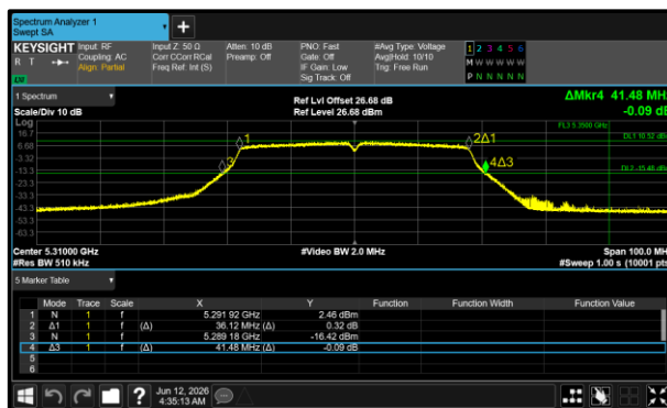
Figure 461 - 802.11n HT40 Minimum 99% OBW
