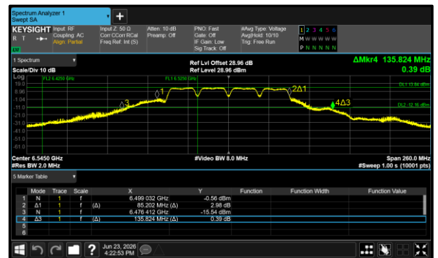
Figure 230 - 802.11a80 SP Maximum 26 dB EBW
