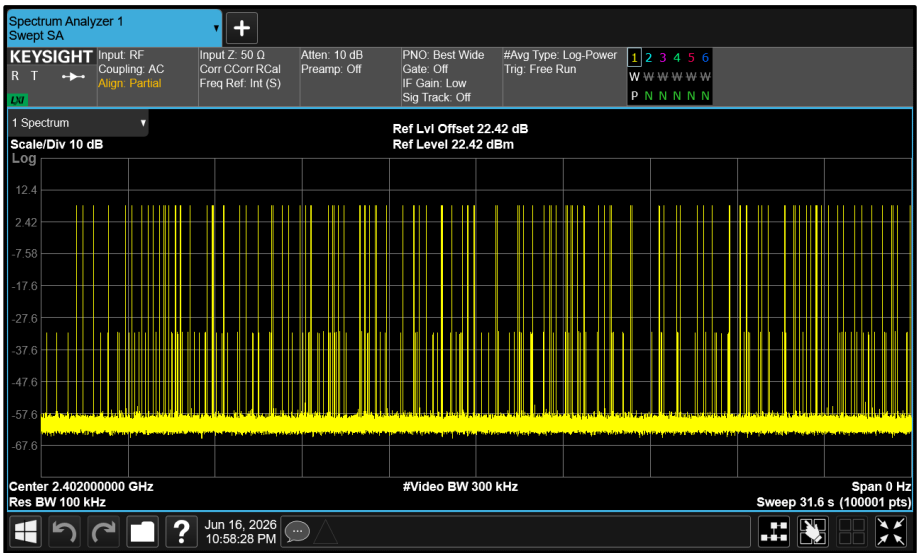
Figure 1 - GFSK - 2402 MHz Accumulated Transmit Time
