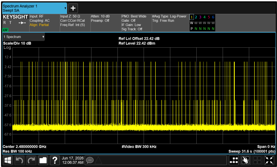
Figure 12 - GFSK - 2480 MHz Accumulated Transmit Time
