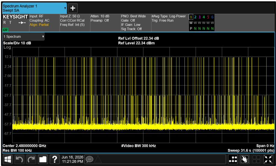
Figure 6 - GFSK - 2480 MHz Accumulated Transmit Time
