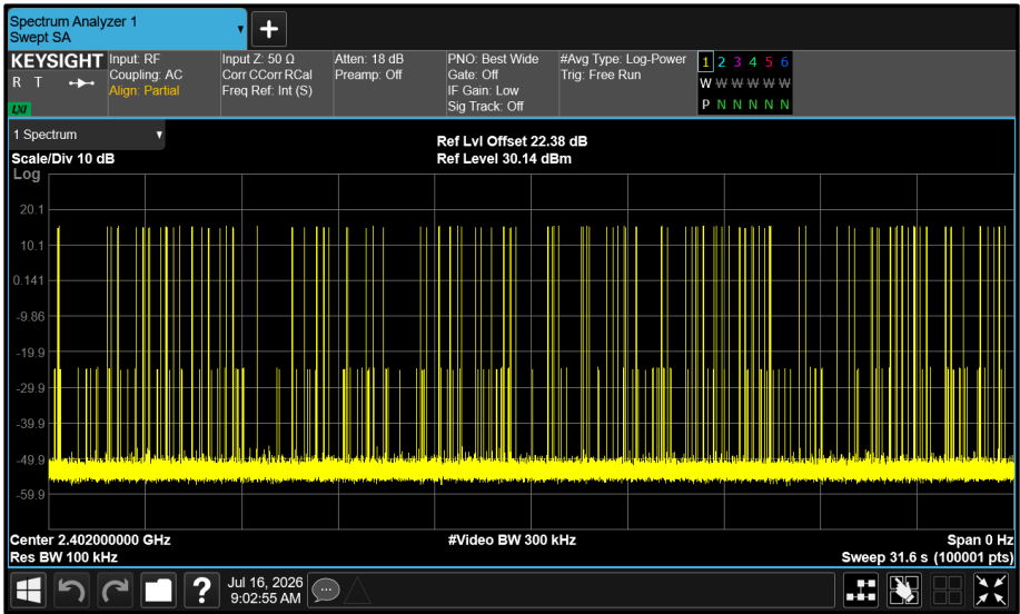
Figure 13 - GFSK - 2402 MHz Accumulated Transmit Time
