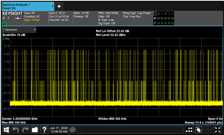
Figure 11 - GFSK - 2402 MHz Accumulated Transmit Time
