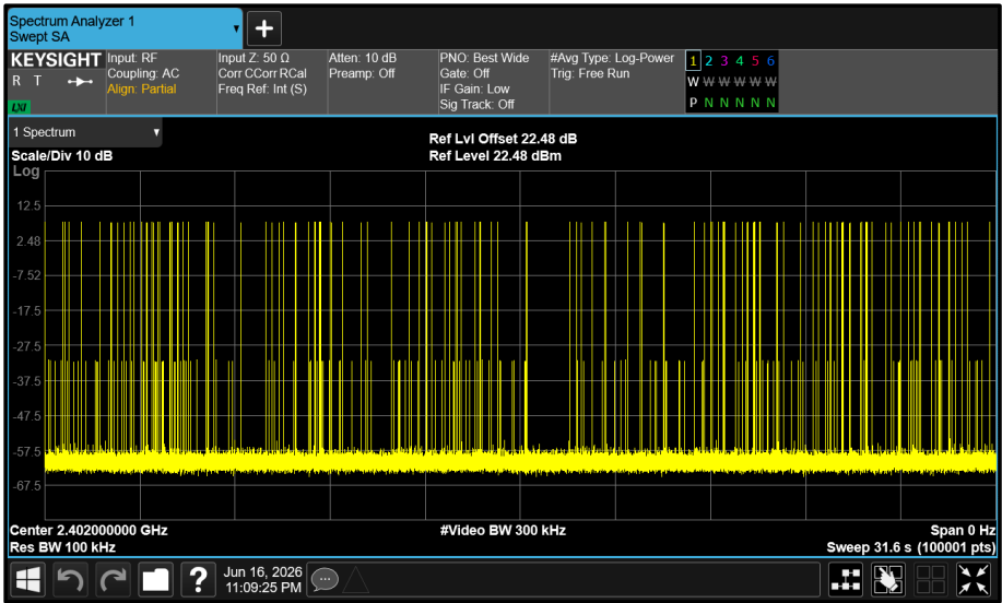
Figure 3 - GFSK - 2402 MHz Accumulated Transmit Time
