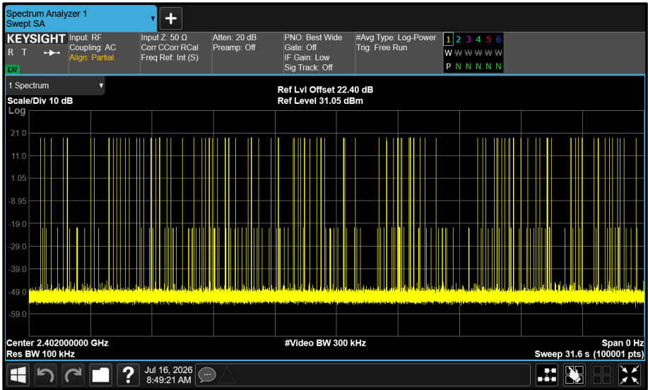
Figure 9 - GFSK - 2402 MHz Accumulated Transmit Time
