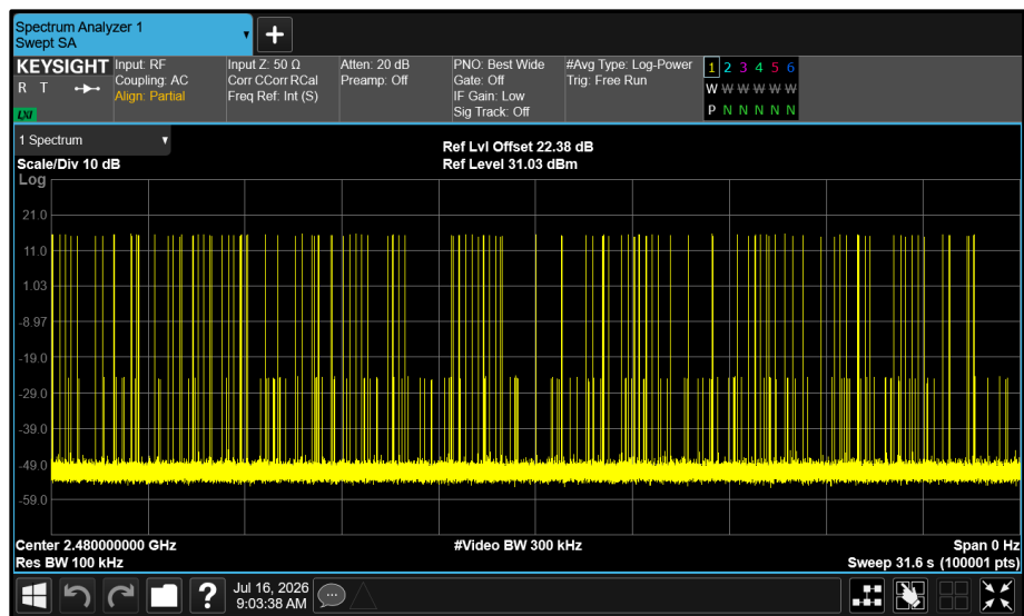
Figure 14 - GFSK - 2480 MHz Accumulated Transmit Time
