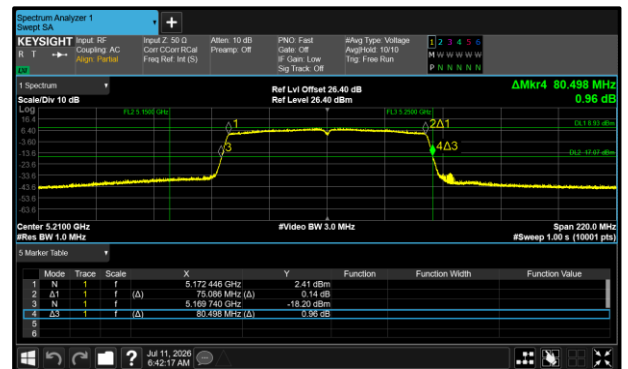
Figure 359 - 802.11ac VHT80 Maximum 26 dB EBW
