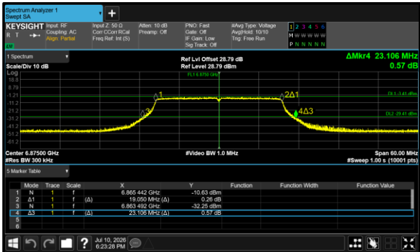
Figure 38- 802.11ax HE20 SU LPI Maximum 26 dB EBW
