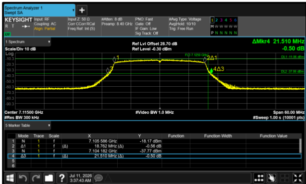
Figure 41- 802.11ax HE20 SU VLP Minimum 26 dB EBW
