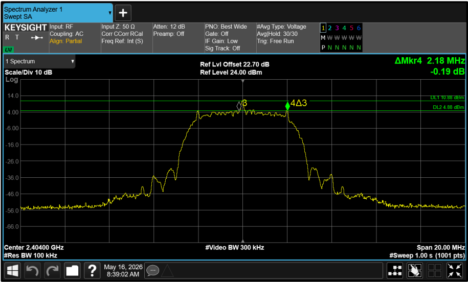
Figure 418 - Core 1 (B) 2404 MHz (CH2) 6 dB Bandwidth
