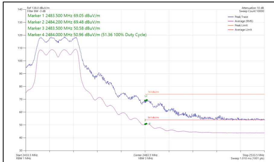
Figure 136 - 802.11g, CDD, Core 0-1 - 2447 MHz Band Edge Frequency 2483.5 MHz
