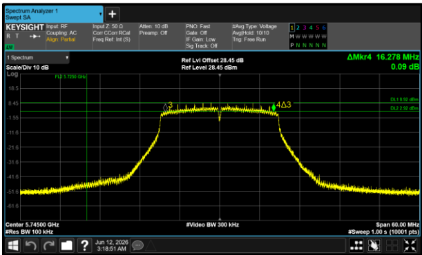
Figure 92 - 802.11n HT20 Maximum 6 dB EBW
