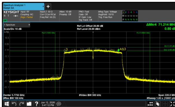
Figure 29 - 802.11ac VHT80 Minimum 6 dB EBW
