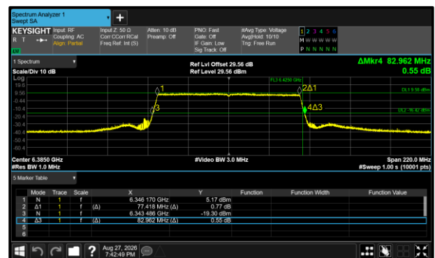
Figure 350 - 802.11ax HE80 SU SP Maximum 26 dB EBW
