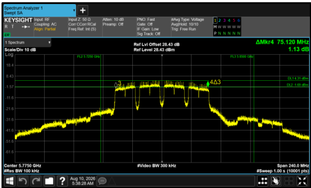
Figure 451 - 802.11a80 Maximum 6 dB EBW
