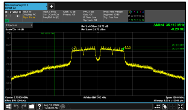
Figure 407 - 802.11a40 Maximum 6 dB EBW
