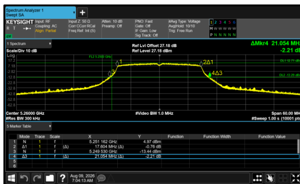
Figure 452 - 802.11n HT20 Minimum 26 dB EBW
