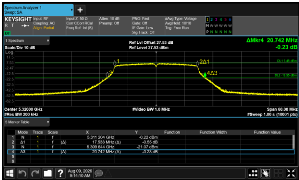
Figure 602 - 802.11ac VHT20 Minimum 26 dB EBW
