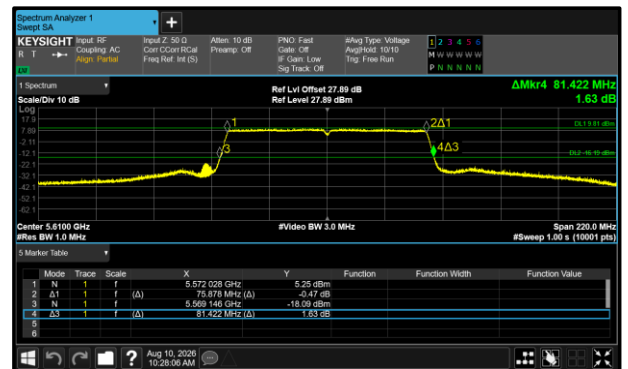
Figure 607 - 802.11ac VHT80 Maximum 26 dB EBW
