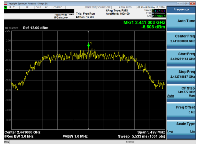
Plot 7-95. Power Spectral Density Plot Antenna WF7 (Bluetooth (HDR4), 4 Mbps, iPA – Ch. 38)
