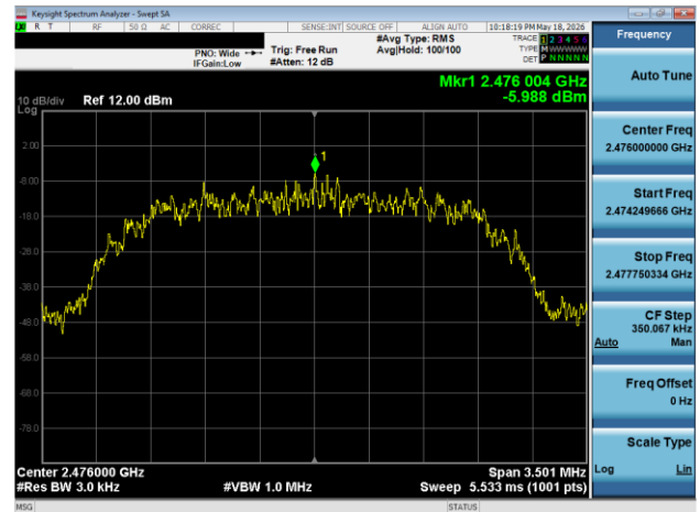
Plot 7-132. Power Spectral Density Plot TxBF Antenna WF7 (Bluetooth (HDR4), 4 Mbps, iPA - Ch. 73)
