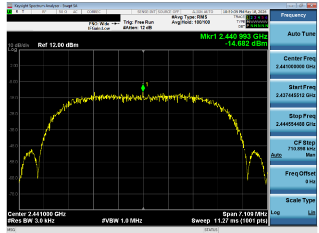
Plot 7-83. Power Spectral Density Plot Antenna WF8 (Bluetooth (XHDRPM6), 6 Mbps, iPA - Ch. 38)
