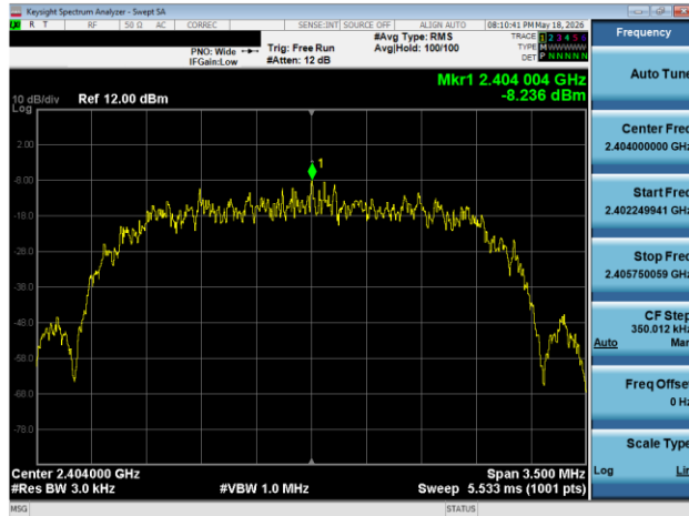
Plot 7-127. Power Spectral Density Plot TxBF Antenna WF8 (Bluetooth (HDR4), 4 Mbps, iPA - Ch. 1)
