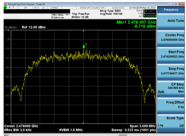
Plot 7-66. Power Spectral Density Plot Antenna WF8 (Bluetooth (HDR4), 4 Mbps, iPA – Ch. 73)
