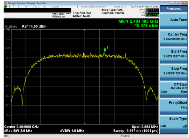
Plot 7-106. Power Spectral Density Plot Antenna WF7 (Bluetooth (HDRPS2), 2Mbps, iPA – Ch. 1)
