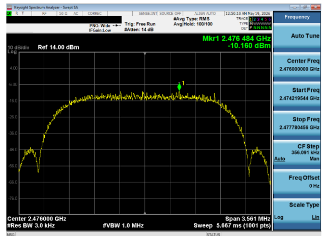
Plot 7-108. Power Spectral Density Plot Antenna WF7 (Bluetooth (HDRPS2), 2Mbps, iPA – Ch. 73)
