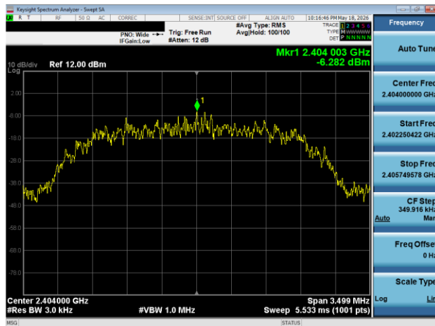
Plot 7-128. Power Spectral Density Plot TxBF Antenna WF7 (Bluetooth (HDR4), 4 Mbps, iPA - Ch. 1)
