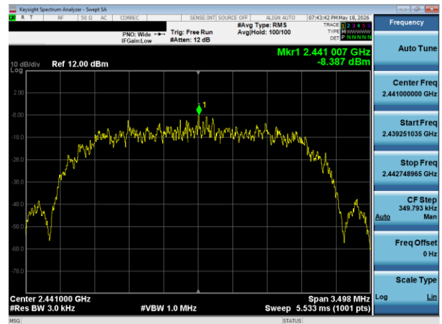
Plot 7-65. Power Spectral Density Plot Antenna WF8 (Bluetooth (HDR4), 4 Mbps, iPA – Ch. 38)
