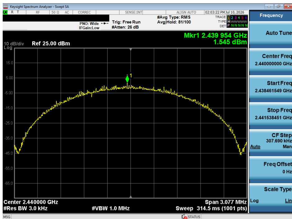
Plot 7-77. Power Spectral Density Plot Antenna WF8 (Bluetooth (LE), 2Mbps, ePA – Ch. 17)
