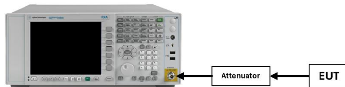
Figure 7-5. Test Instrument & Measurement Setup
