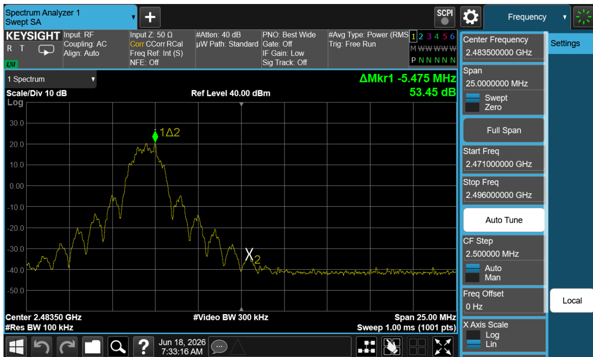
Plot 7-126. Band Edge Plot Antenna WF7 (BTCSM1_LE2M 2.0, ePA – Ch. 36)
