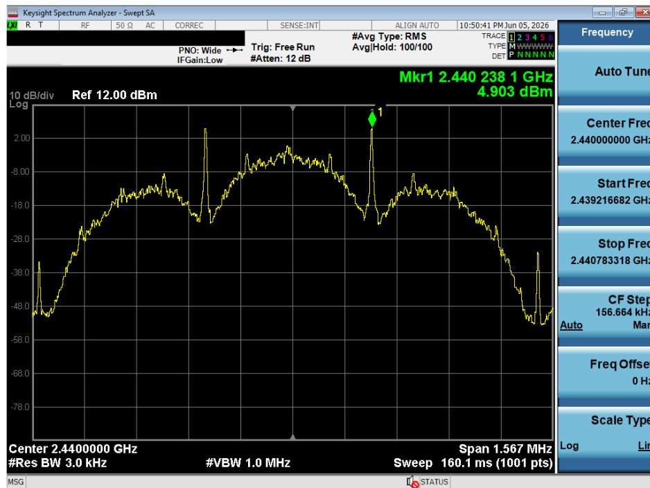
Plot 7-68. Power Spectral Density Plot Antenna WF7 (Bluetooth (LE), 125kbps, iPA – Ch. 17)
