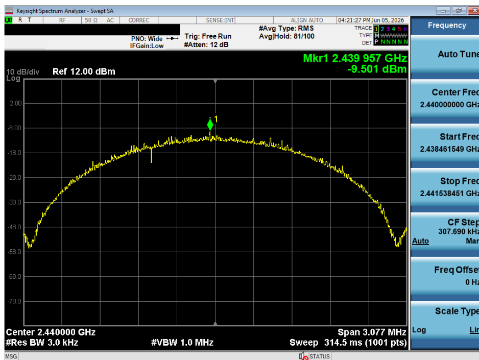
Plot 7-79. Power Spectral Density Plot Antenna WF8 (Bluetooth (LE), 2Mbps, iPA – Ch. 17)
