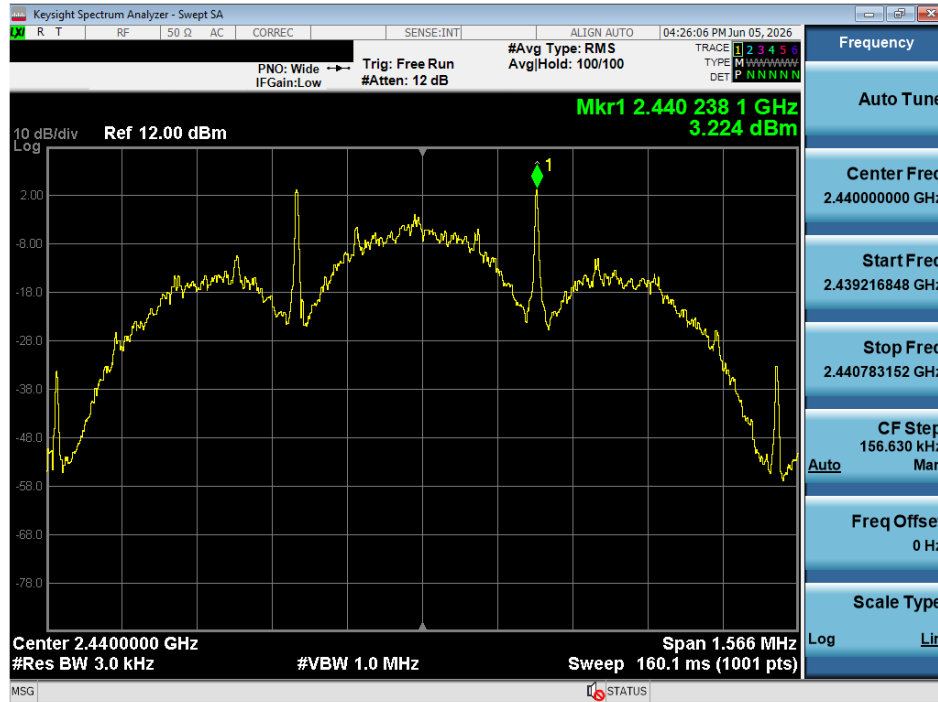
Plot 7-67. Power Spectral Density Plot Antenna WF8 (Bluetooth (LE), 125kbps, iPA – Ch. 17)
