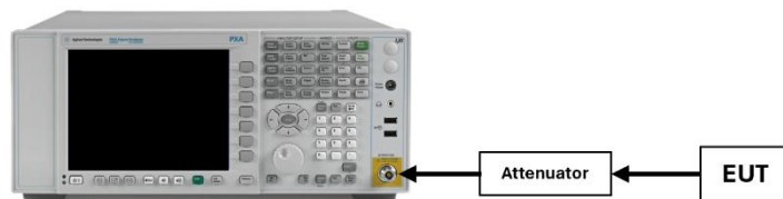
Figure 7-6. Test Instrument & Measurement Setup
