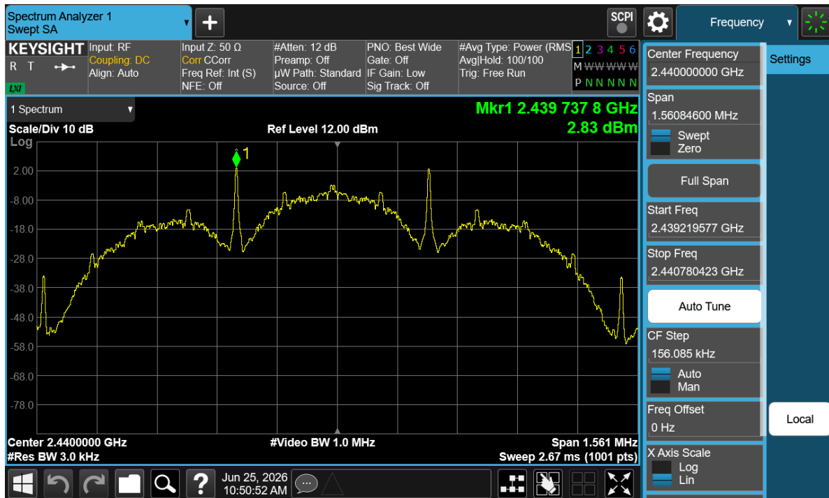
Plot 7-66. Power Spectral Density Plot Antenna WF7 (Bluetooth (LE), 125kbps, ePA – Ch. 17)
