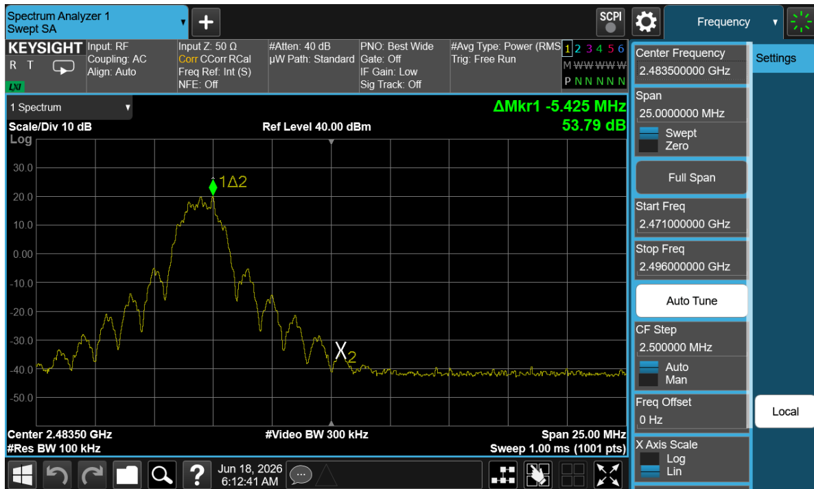
Plot 7-110. Band Edge Plot Antenna WF8 (BTCM1_LE2M 2.0, ePA – Ch. 36)
