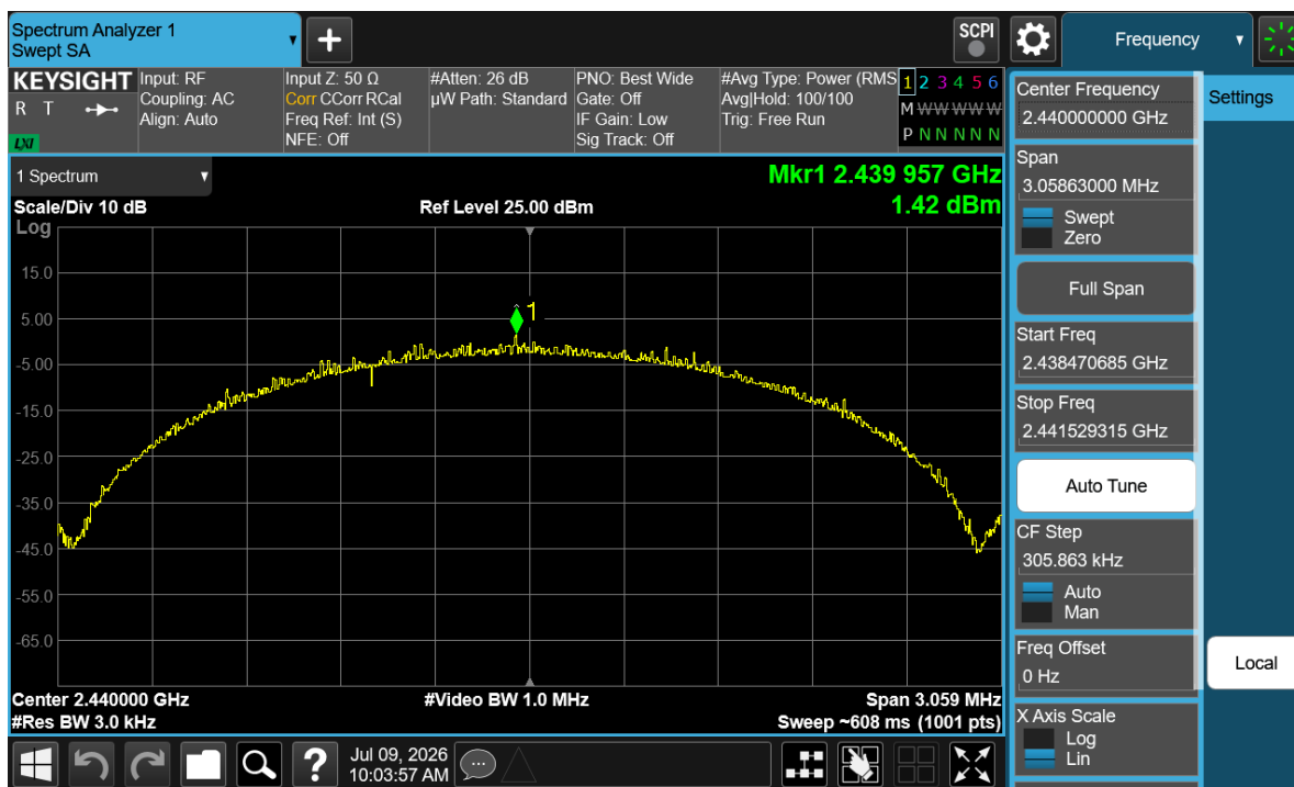
Plot 7-86. Power Spectral Density Plot Antenna WF7 (BTCSM1_LE2M, ePA – Ch. 17)
