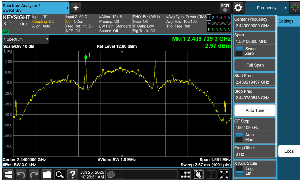
Plot 7-65. Power Spectral Density Plot Antenna WF8 (Bluetooth (LE), 125kbps, ePA – Ch. 17)
