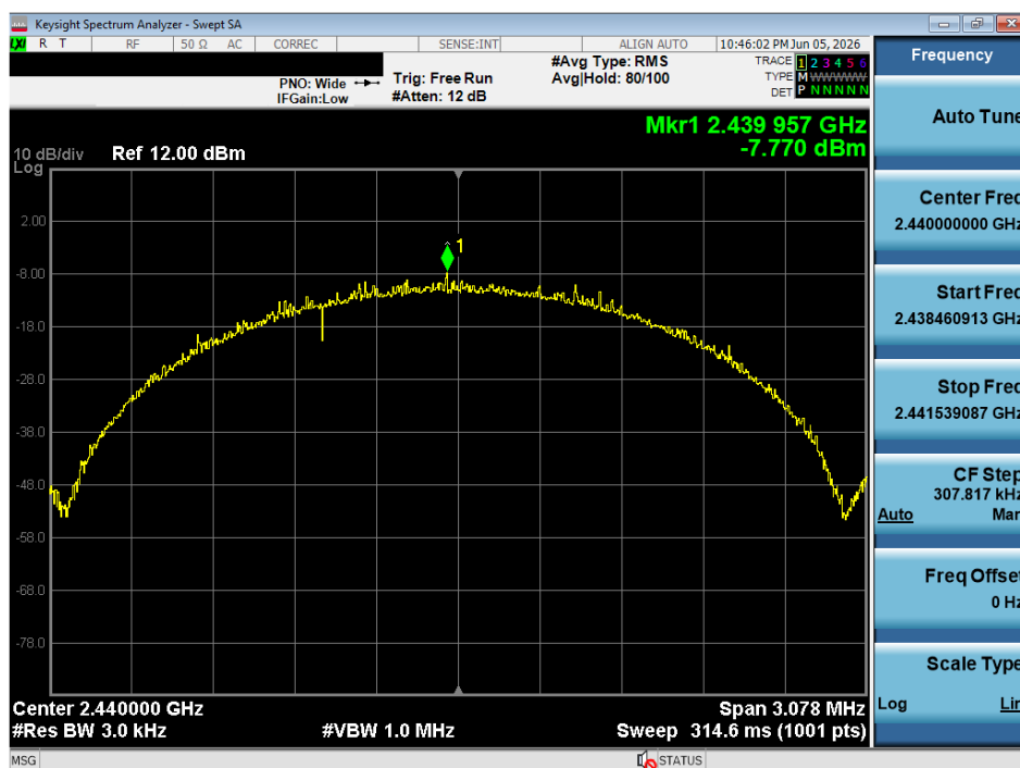
Plot 7-80. Power Spectral Density Plot Antenna WF7 (Bluetooth (LE), 2Mbps, iPA – Ch. 17)
