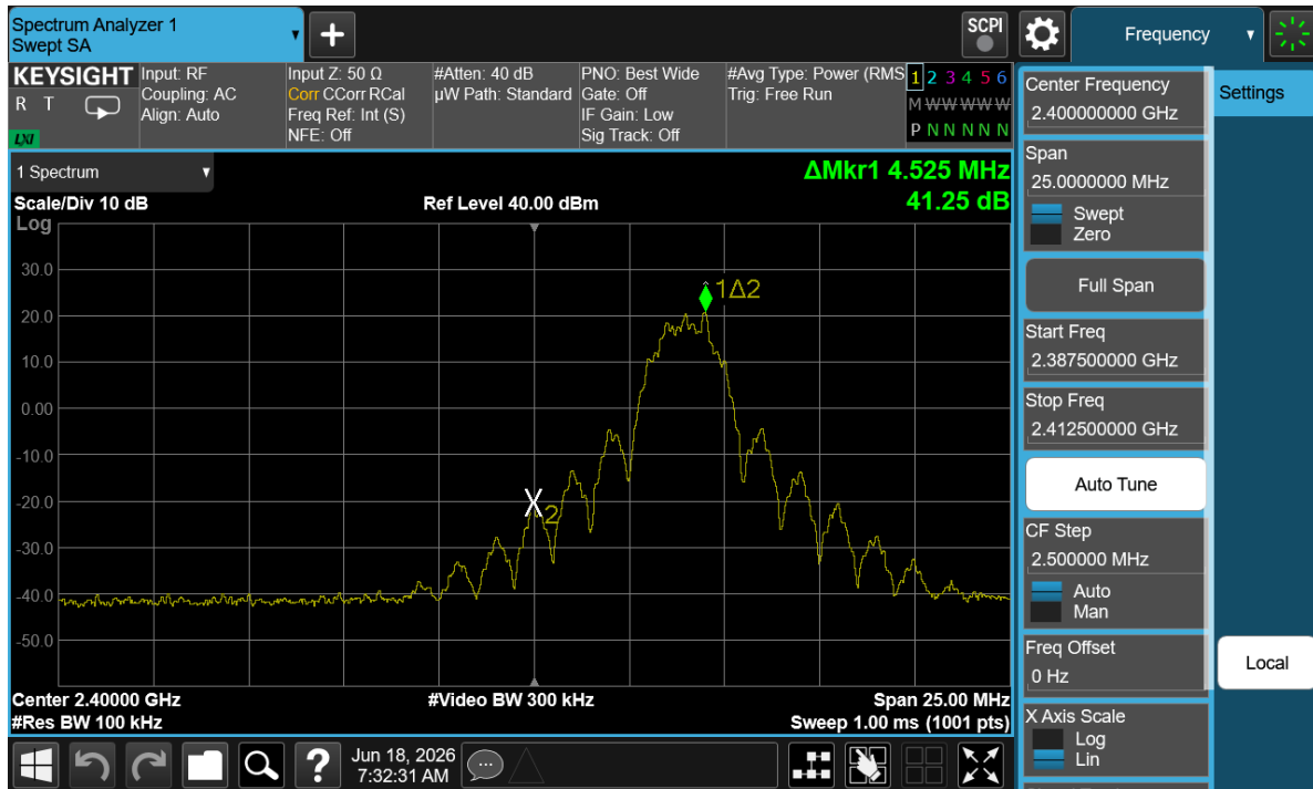
Plot 7-125. Band Edge Plot Antenna WF7 (BTCSM1_LE2M 2.0, ePA – Ch. 0)
