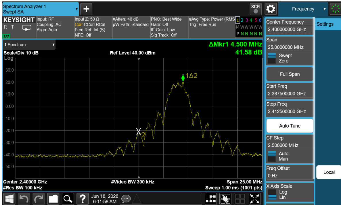
Plot 7-109. Band Edge Plot Antenna WF8 (BTCM1_LE2M 2.0, ePA – Ch. 0)
