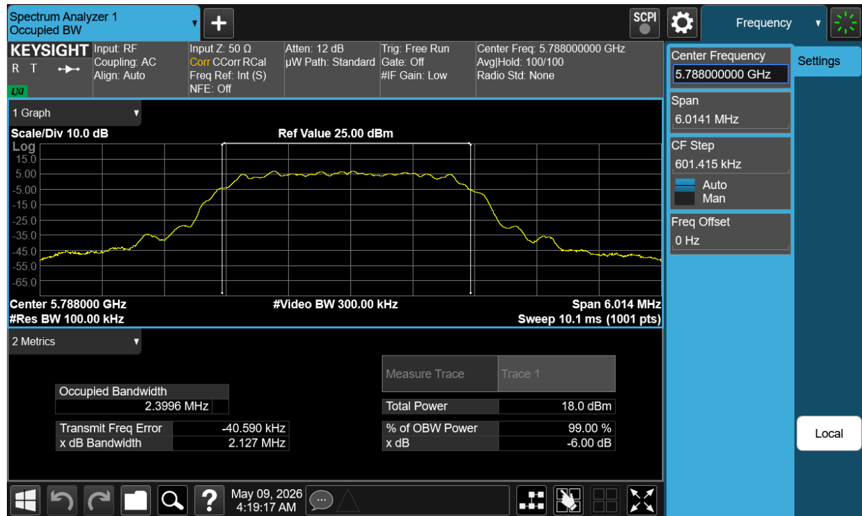
Plot 7-104. 6 dB BW & 99% OBW Antenna WF5B (NB UNII HDT6, ePA- 5788 MHz)
