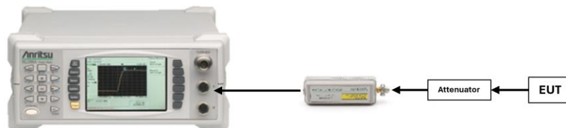
Figure 7-3. Test Instrument & Measurement Setup
