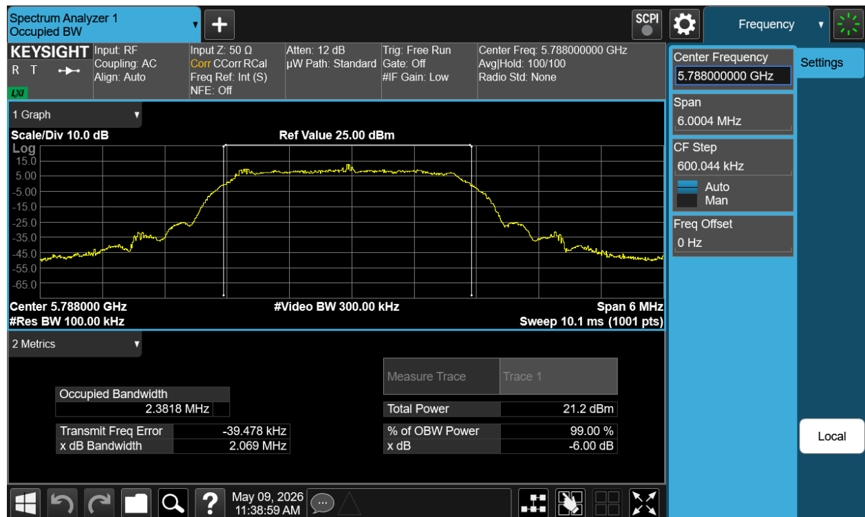
Plot 7-110. 6 dB BW & 99% OBW Antenna WF8 (NB UNII HDRPS2, ePA – 5788 MHz)
