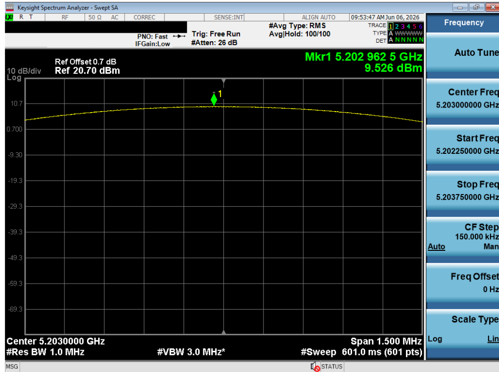
Plot 7-120. PSD Antenna WF5T (NB UNII LE1M, ePA – 5203 MHz)
