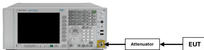
Figure 7-4. Test Instrument & Measurement Setup
