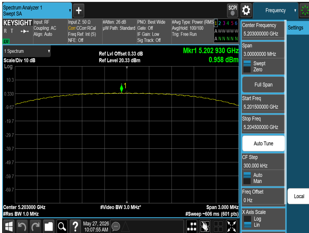
Plot 7-129. PSD Antenna WF5T (NB UNII HDRPS2, iPA – 5203 MHz)
