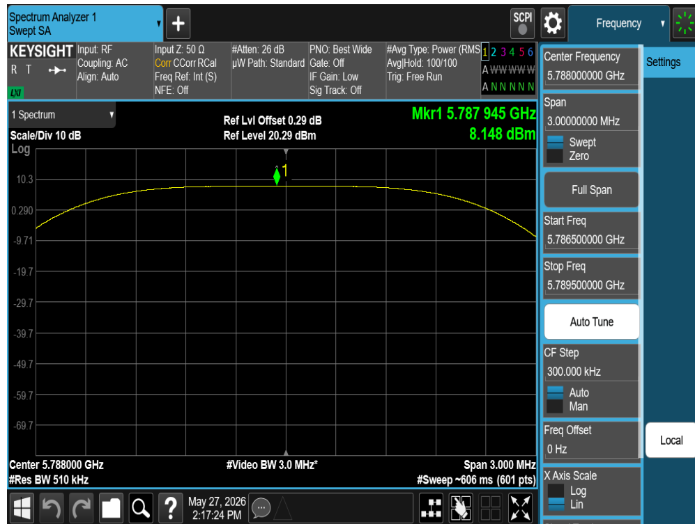
Plot 7-474. PSD TxBF Diversity Antenna WF5T (NB UNII HDT4, ePA – 5788 MHz)
