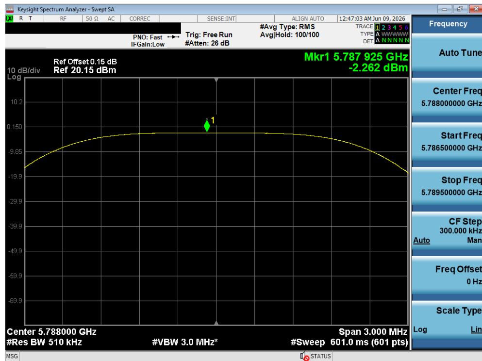
Plot 7-473. PSD Tx BF Diversity Antenna WF8 (NB UNII HDT2, iPA – 5788 MHz)
