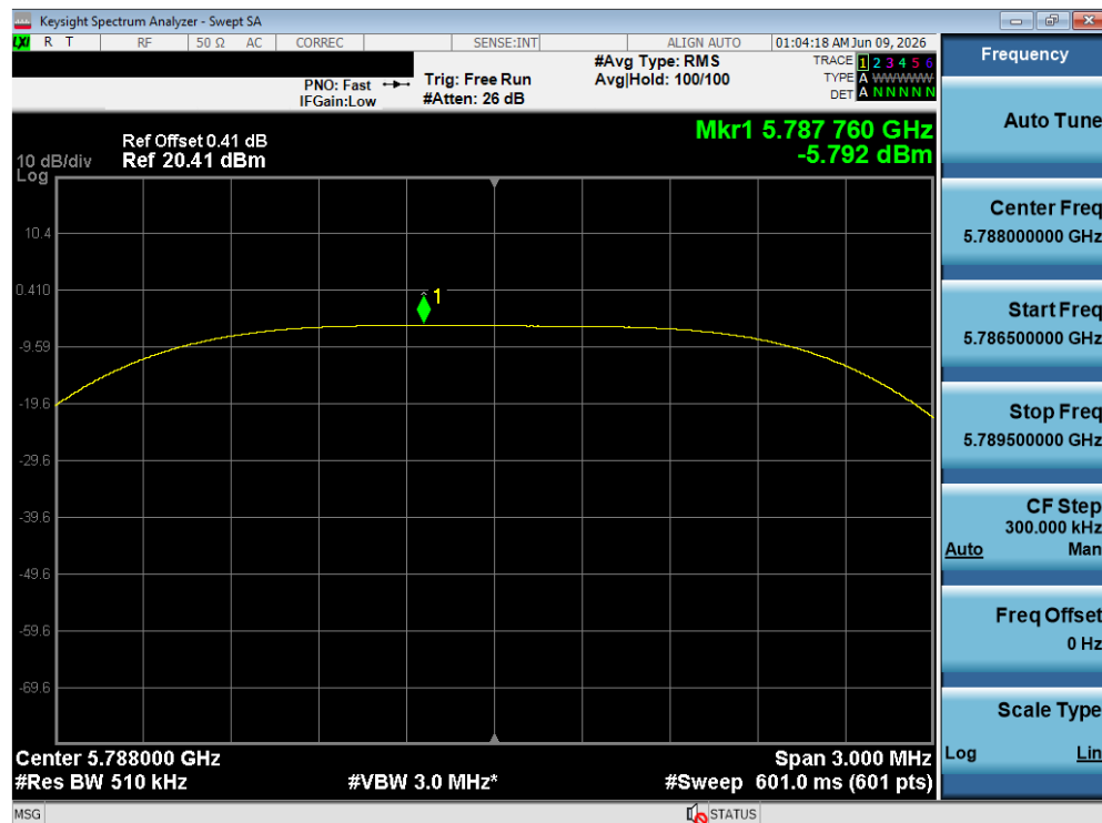
Plot 7-481. PSD TxBF Diversity Antenna WF8 (NB UNII HDT6, iPA – 5788 MHz)
