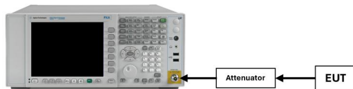
Figure 7-4. Test Instrument & Measurement Setup
