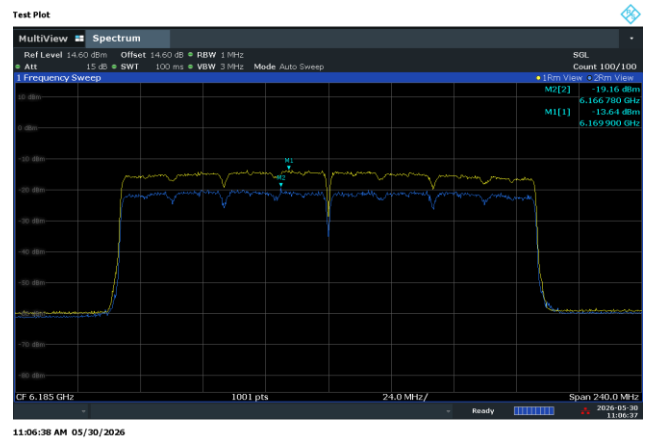
Plot 7-310. 160 MHz Bandwidth – 6185 MHz Antenna WF5B
