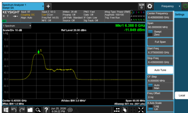
Plot 7-266 PSD SDM Primary Antenna WF5T (40 MHz BW 802.11be(RU) RU52 Index37 - Ch.91)
