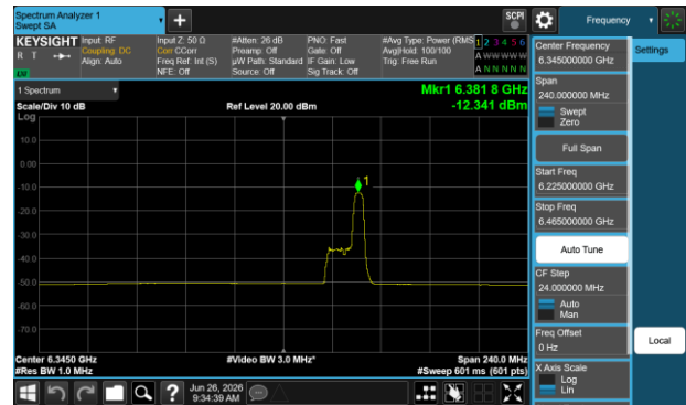
Plot 7-272 PSD SDM Primary Antenna WF5B (160 MHz BW 802.11be(RU) RU52 Index44 - Ch.79)
