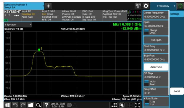
Plot 7-270 PSD SDM Primary Antenna WF5B (40 MHz BW 802.11be(RU) RU52 Index37 - Ch.91)
