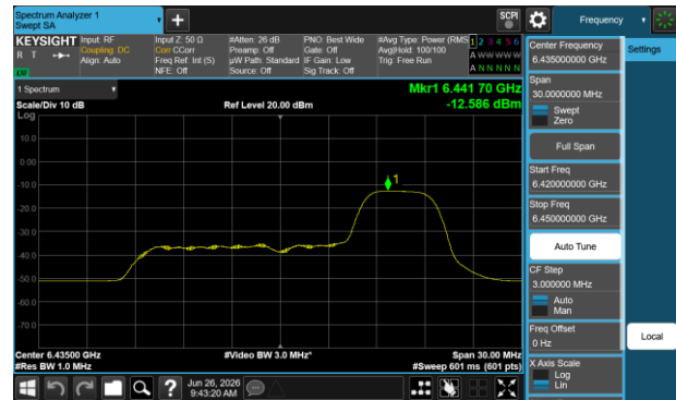
Plot 7-291 PSD SDM Primary Antenna WF5B (20 MHz BW 802.11be(RU) RU52 Index40 - Ch.97)
