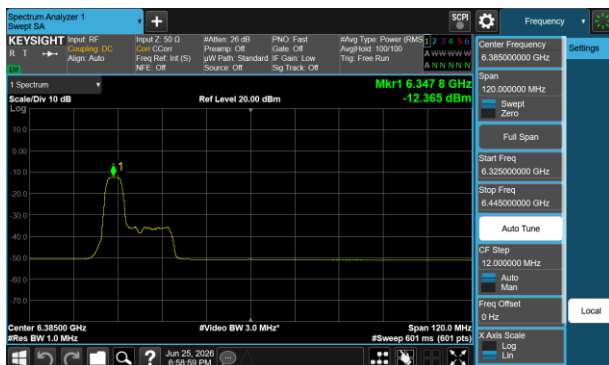
Plot 7-355 PSD SDM Diversity Antenna WF5T (80 MHz BW 802.11be(RU) RU52 Index37 - Ch.87)
