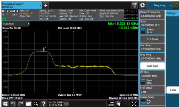
Plot 7-397 PSD SDM Diversity Antenna WF5T (20 MHz BW 802.11be(RU) RU52 Index37 - Ch.117)
