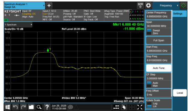
Plot 7-335 PSD SDM Primary Antenna WF5B (20 MHz BW 802.11be(RU) RU52 Index37 - Ch.189)
