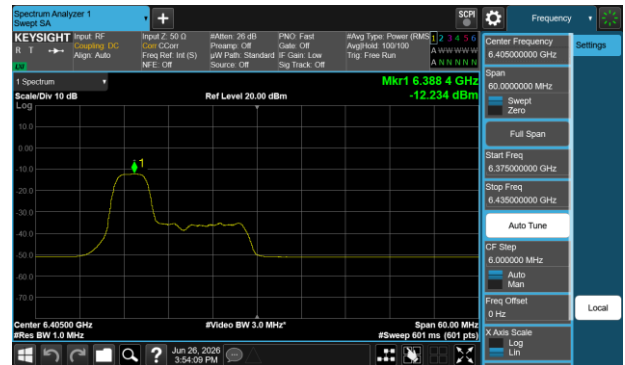
Plot 7-358 PSD SDM Diversity Antenna WF8 (40 MHz BW 802.11be(RU) RU52 Index37 - Ch.91)
