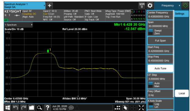
Plot 7-379 PSD SDM Diversity Antenna WF8 (20 MHz BW 802.11be(RU) RU52 Index37 - Ch.97)
