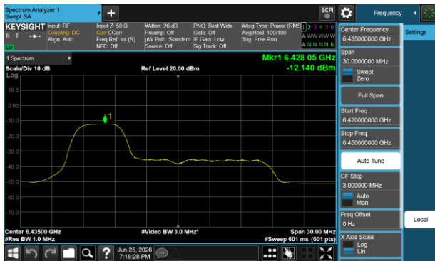
Plot 7-375 PSD SDM Diversity Antenna WF5T (20 MHz BW 802.11be(RU) RU52 Index37 - Ch.97)
