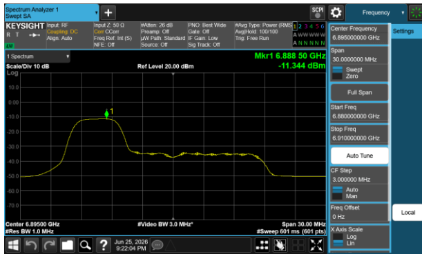
Plot 7-331 PSD SDM Primary Antenna WF5T (20 MHz BW 802.11be(RU) RU52 Index37 - Ch.189)
