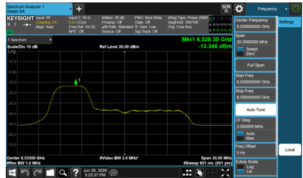
Plot 7-401 PSD SDM Diversity Antenna WF8 (20 MHz BW 802.11be(RU) RU52 Index37 - Ch.117)
