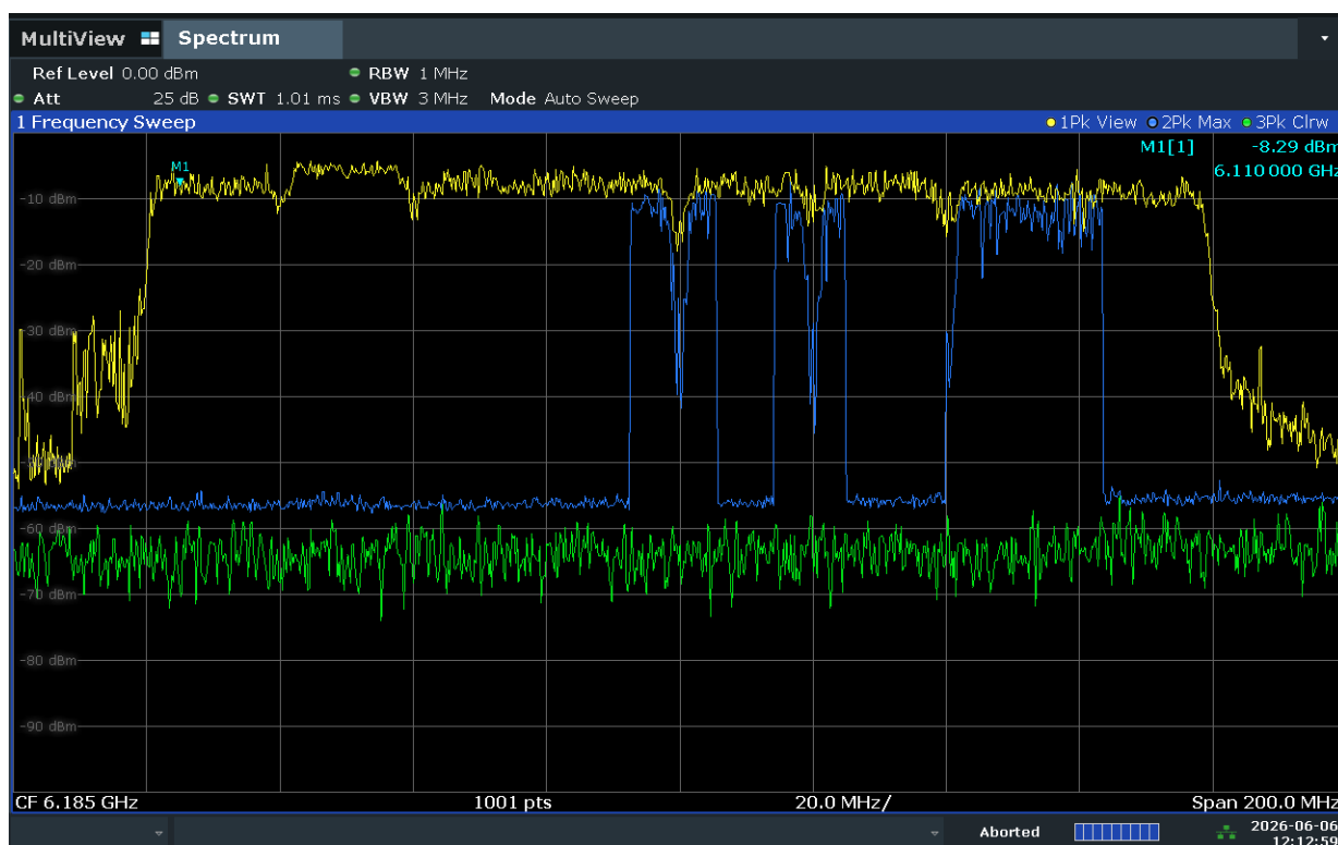
Plot 7-782. 160 MHz Bandwidth, AWGN Signal Injected – 6110 MHz
