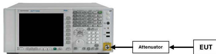
Figure 7-5. Test Instrument & Measurement Setup
