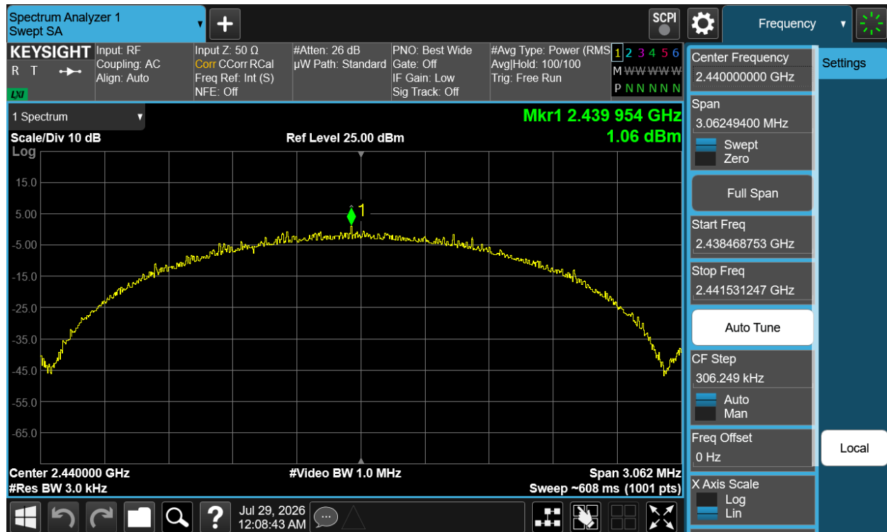
Plot 7-77. Power Spectral Density Plot Antenna 3A (Bluetooth (LE), 2Mbps, ePA – Ch. 17)
