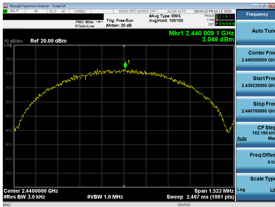
Plot 7-81. Power Spectral Density Plot Antenna 3A (BTCSM1_LE1M, ePA – Ch. 17)
