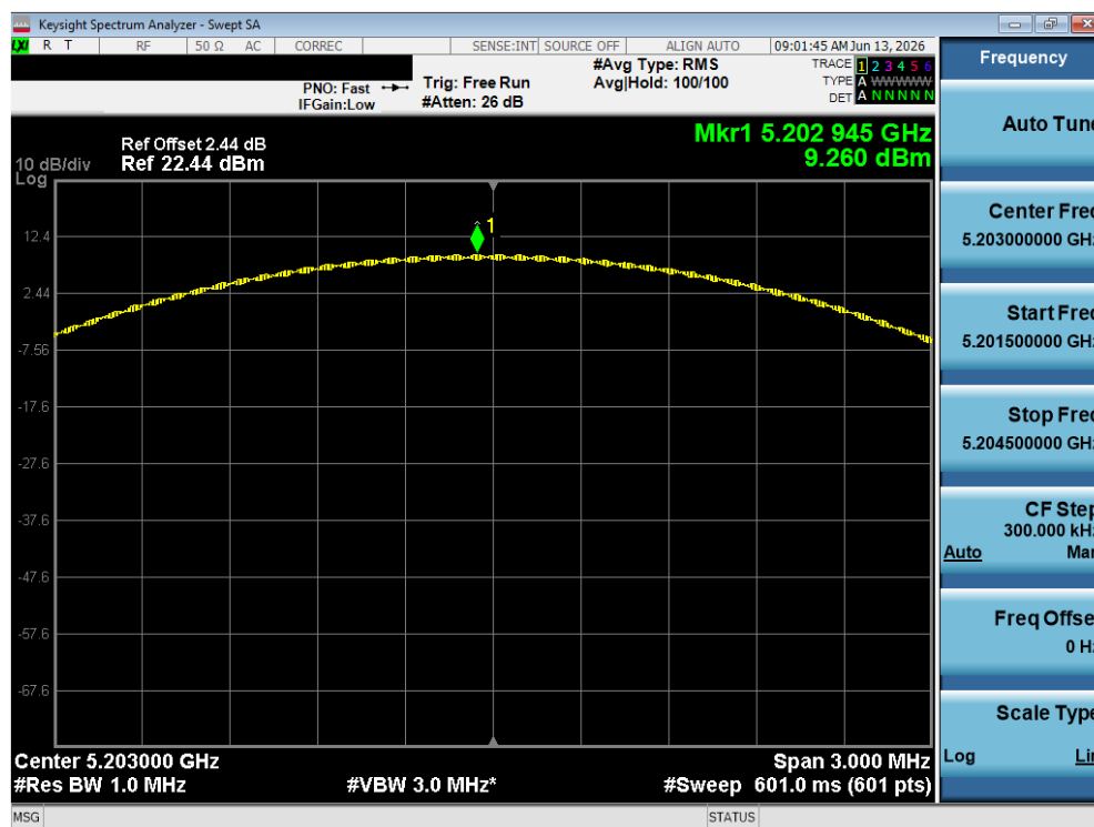
Plot 7-226. PSD Antenna 1B (NB UNII LE2M, ePA – 5203 MHz)
