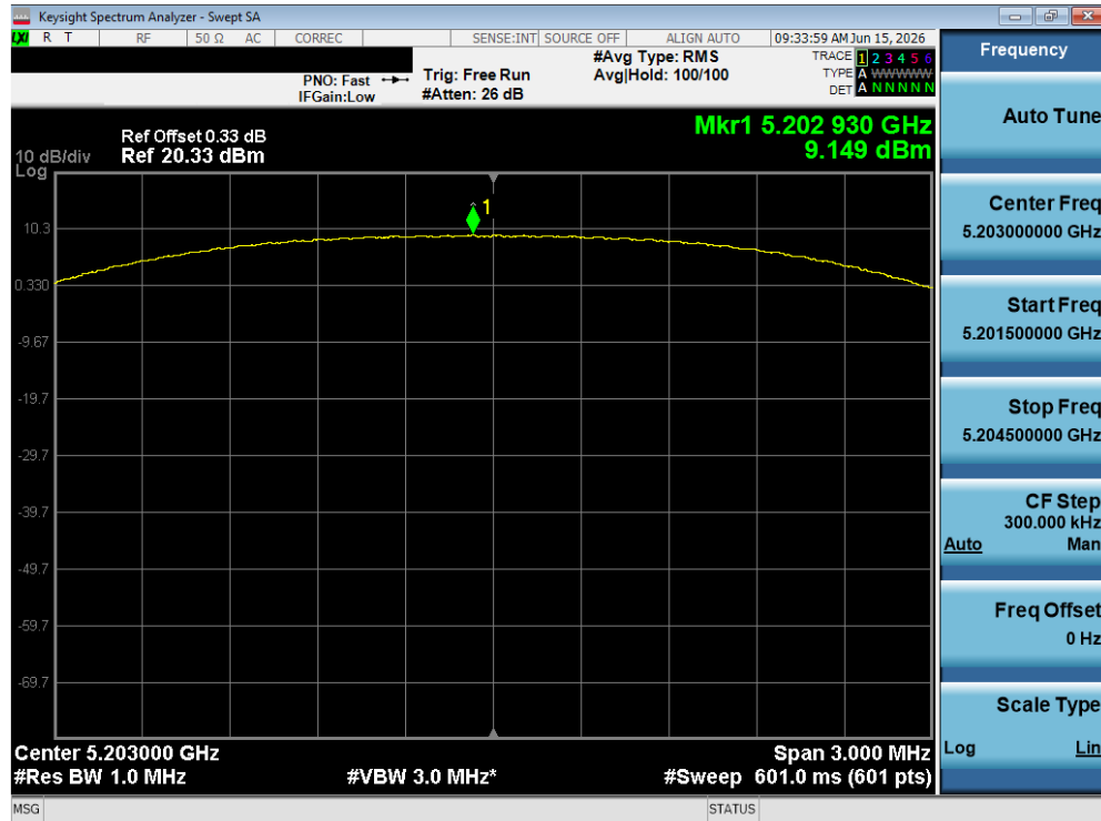
Plot 7-180. PSD Antenna 5B (NB UNII HDRPS2, ePA – 5203 MHz)
