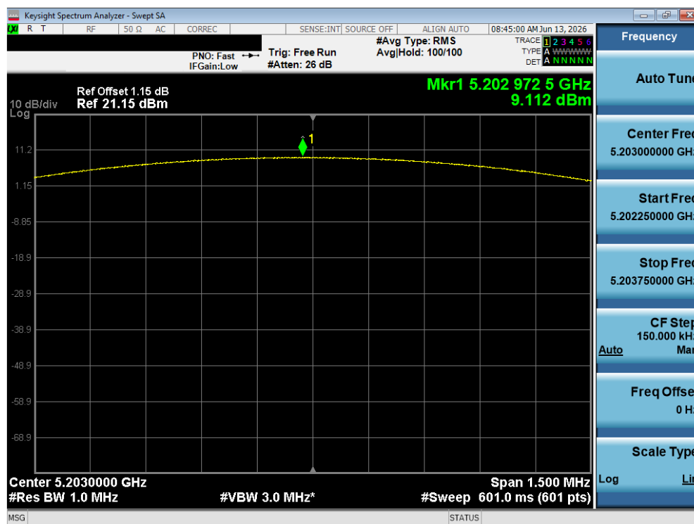
Plot 7-222. PSD Antenna 1B (NB UNII BDR, ePA – 5203 MHz)
