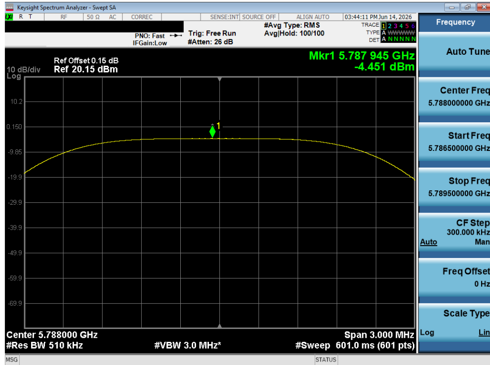
Plot 7-368. PSD TxBF Primary Antenna 5T (NB UNII HDT2, iPA – 5788 MHz)
