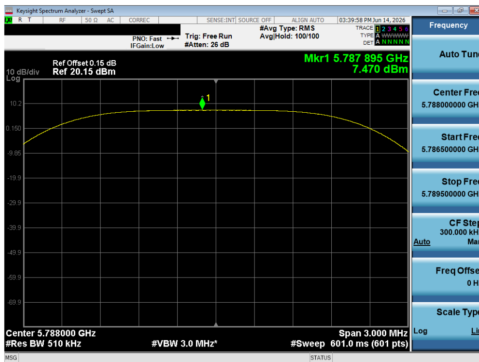
Plot 7-470. PSD TxBF Diversity Antenna 5T (NB UNII HDT2, ePA – 5788 MHz)
