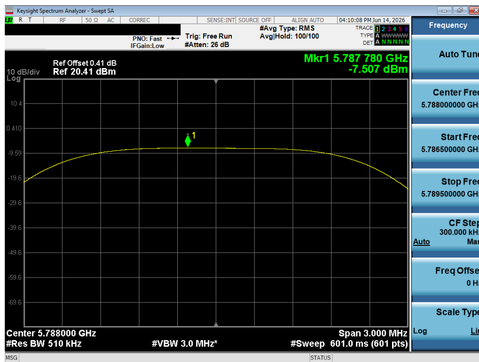
Plot 7-376. PSD TxBF Primary Antenna 5T (NB UNII HDT6, iPA – 5788 MHz)
