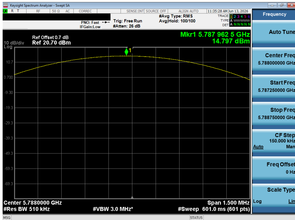
Plot 7-435. PSD TxBF Diversity Antenna 1B (NB UNII LE1M, ePA – 5788 MHz)
