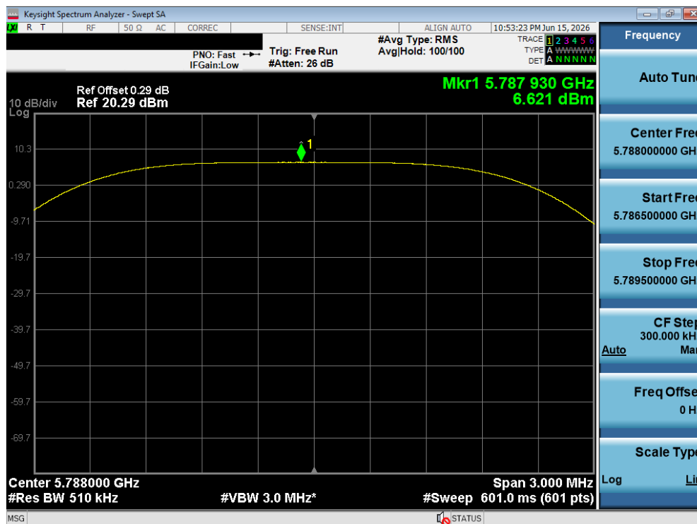
Plot 7-475. PSD TxBF Diversity Antenna 1B (NB UNII HDT4, ePA – 5788 MHz)
