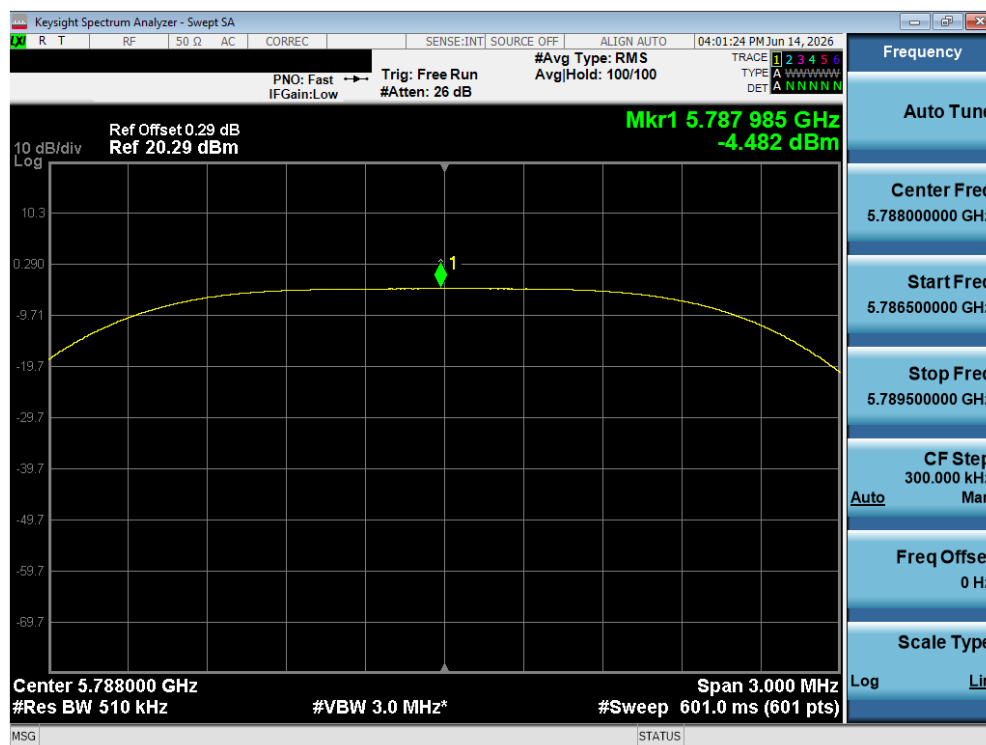
Plot 7-372. PSD TxBF Primary Antenna 5T (NB UNII HDT4, iPA – 5788 MHz)
