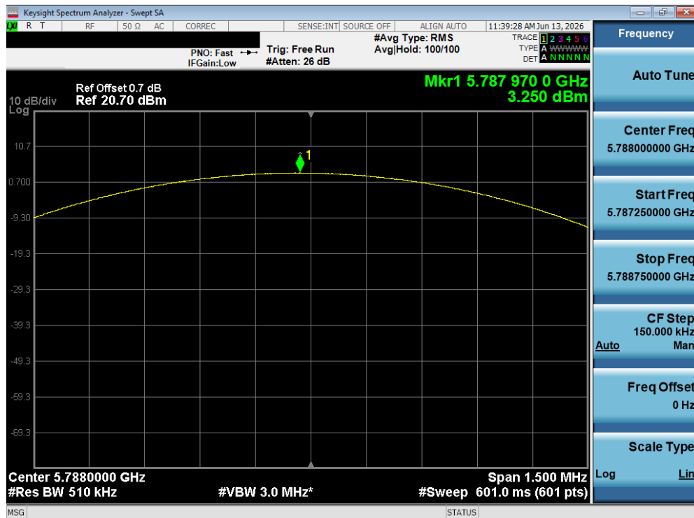
Plot 7-437. PSD TxBF Diversity Antenna 1B (NB UNII LE1M, iPA – 5788 MHz)
