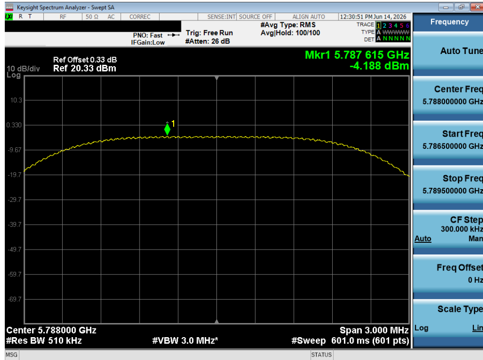
Plot 7-452. PSD TxBF Diversity Antenna 5T (NB UNII HDRPS2, iPA – 5788 MHz)
