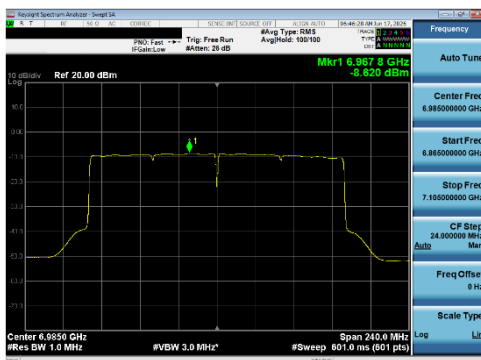
Plot 7-220 PSD SDM Primary Antenna 5T (160 MHz BW 802.11be(SU) - Ch.207)
