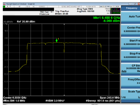
Plot 7-132 PSD Antenna 5B (160 MHz BW 802.11be(SU) - Ch.111)
