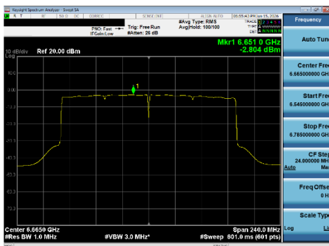
Plot 7-188 PSD CDD Primary Antenna 5T (160 MHz BW 802.11be(SU) - Ch.143)
