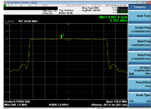
Plot 7-191 PSD CDD Primary Antenna 5B (80 MHz BW 802.11be(SU) - Ch.151)
