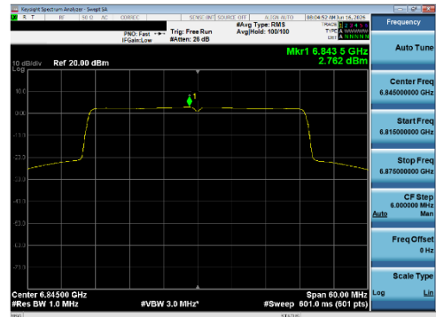
Plot 7-190 PSD CDD Primary Antenna 5B (40 MHz BW 802.11be(SU) - Ch.179)
