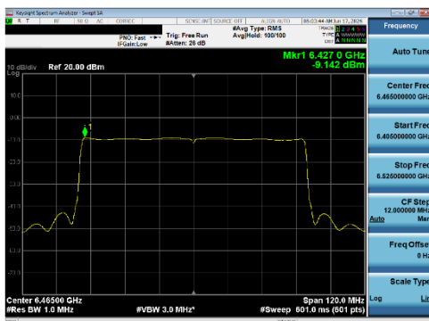
Plot 7-203 PSD SDM Primary Antenna 5T (80 MHz BW 802.11be(SU) - Ch.103)
