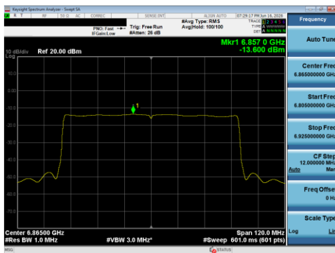
Plot 7-115 PSD SDM Primary Antenna 5T (80 MHz BW 802.11be(SU) - Ch.183)
