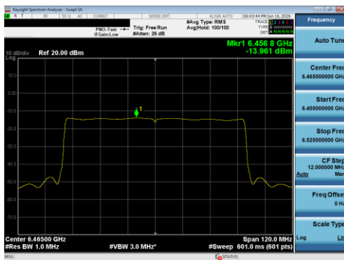
Plot 7-107 PSD SDM Primary Antenna 5T (80 MHz BW 802.11be(SU) - Ch.103)
