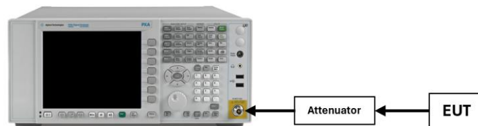
Figure 7-1. Test Instrument & Measurement Setup
