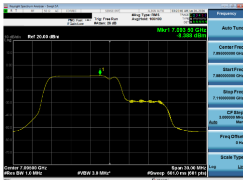
Plot 7-210 PSD Antenna 5B (20 MHz BW 802.11be(RU) RU106+26 Index82 - Ch.229)
