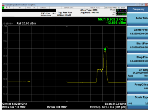
Plot 7-308 PSD SDM Primary Antenna 5T (160 MHz BW 802.11be(RU) RU52 Index52 - Ch.175)
