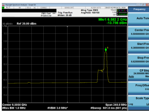
Plot 7-286 PSD SDM Primary Antenna 5T (160 MHz BW 802.11be(RU) RU52 Index52 - Ch.111)
