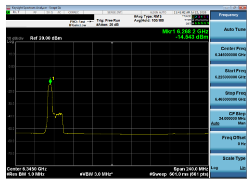
Plot 7-268 PSD SDM Primary Antenna 5B (160 MHz BW 802.11be(RU) RU52 Index37 - Ch.79)
