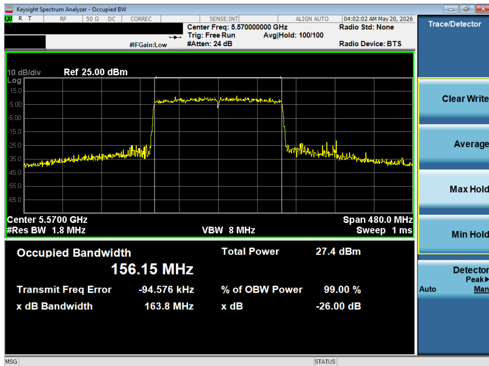
Plot 7-4 26 dB BW & 99% OBW Antenna 5T (160 MHz BW 802.11be(SU) - Ch.114)
