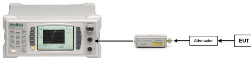
Figure 7-3. Test Instrument & Measurement Setup
