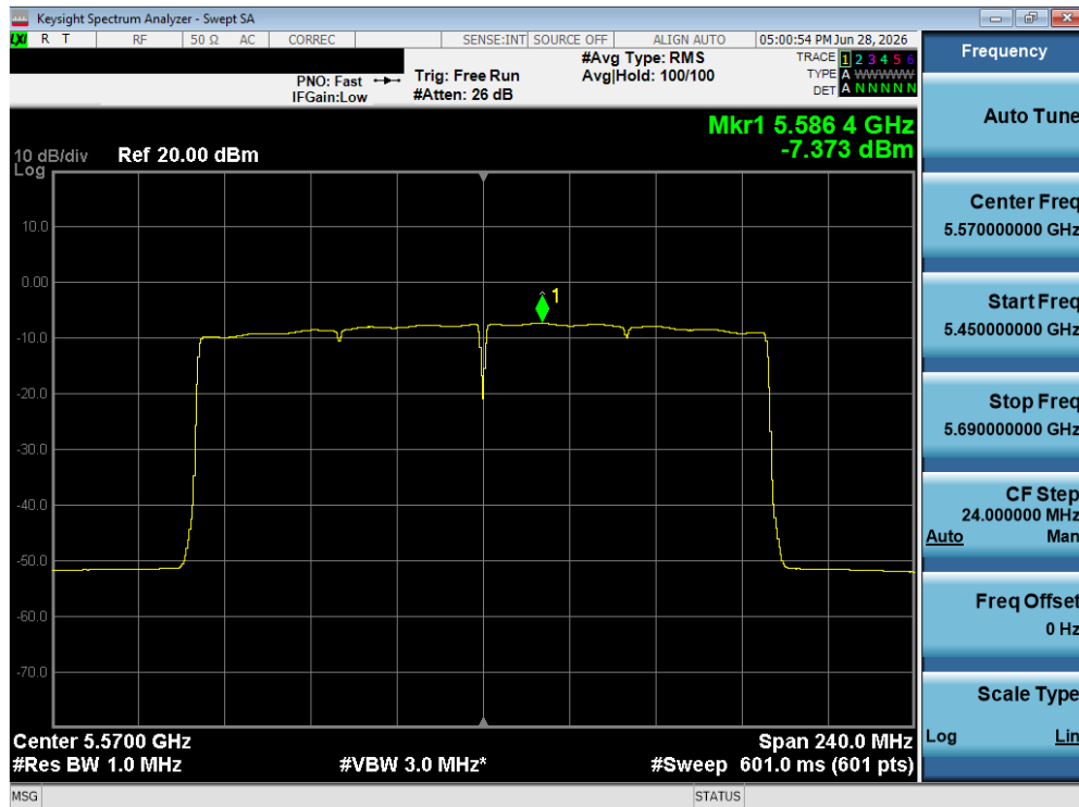
Plot 7-47 PSD Antenna 1B (160 MHz BW 802.11be(SU) - Ch.114)
