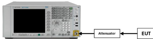
Figure 7-2. Test Instrument & Measurement Setup
