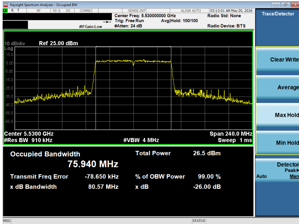
Plot 7-3 26 dB BW & 99% OBW Antenna 5T (80 MHz BW 802.11ac - Ch.106)
