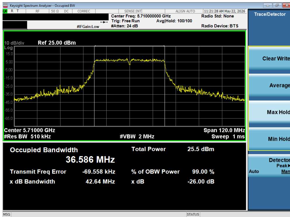
Plot 7-10 26 dB BW & 99% OBW Antenna 1B (40 MHz BW 802.11n - Ch.142)
