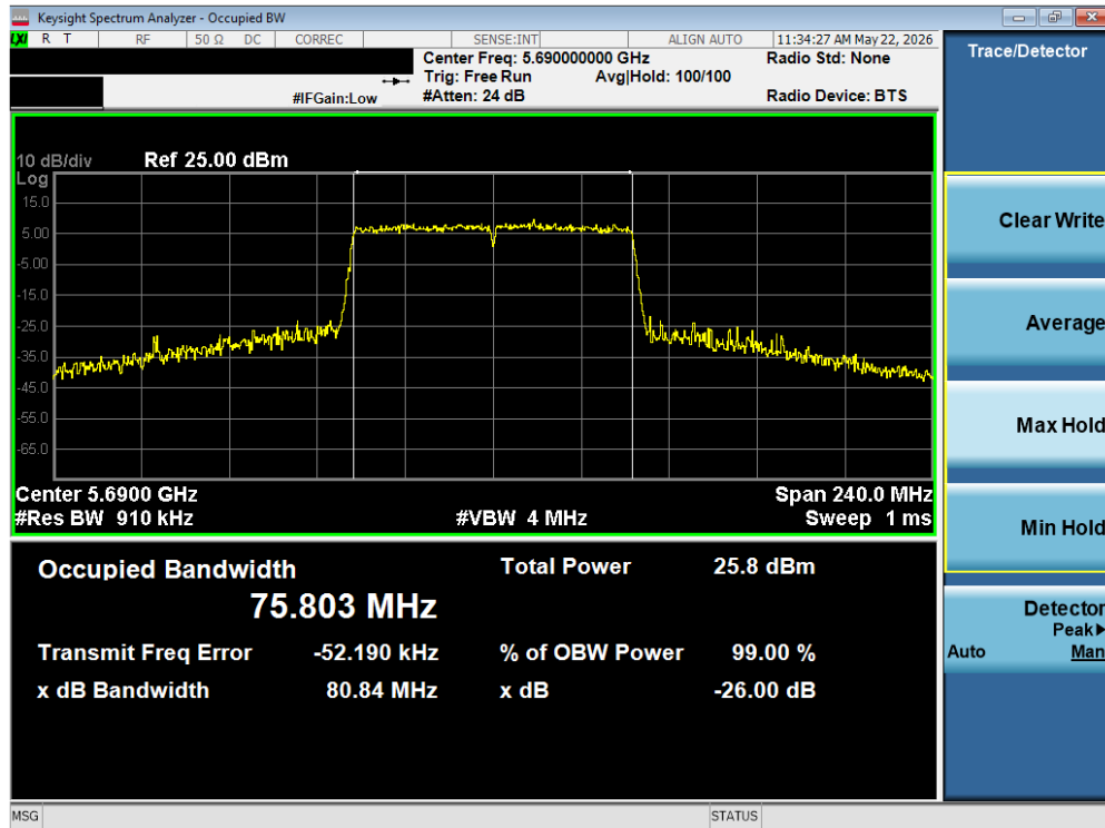
Plot 7-11 26 dB BW & 99% OBW Antenna 1B (80 MHz BW 802.11ac - Ch.138)
