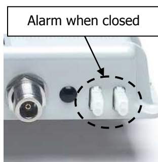
Fig. 16 - External alarms (dry contacts)
