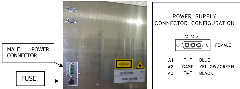
Fig. 27 VDC Connector (TPR922 only)
