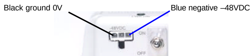
Figure 7 DC Power Connections for Local Unit TFLF
