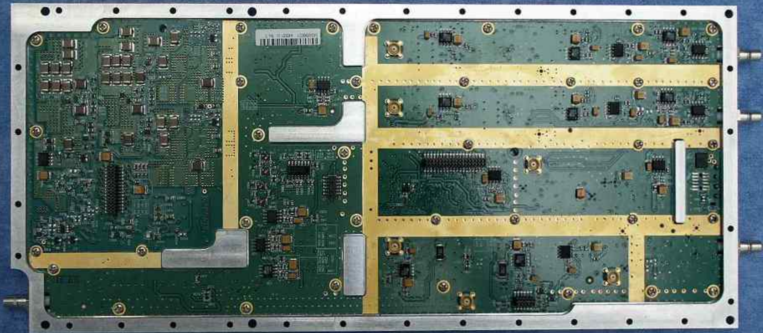
RF Module - Downlink - Bottom
